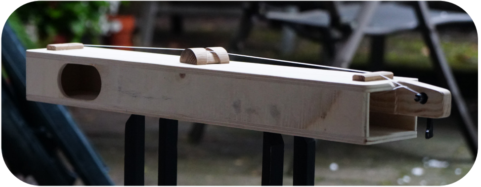
FIG. 35 PROTOTYPE V2 HAS A DYNAMICALLY MOVEABLE BRIDGE TO CHANGE THE PITCH OF THE NOTE WHILE PLAYING
