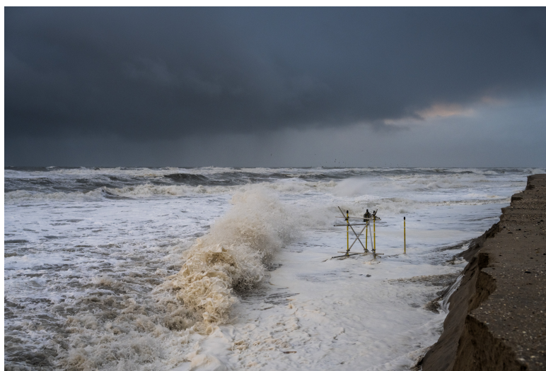
Figure 3.1. Impression of dune erosion at Dune 1 of the field site (Figure 3.2) during storm conditions on January 5, 2022 (Ph. Mischa Keijser). Instruments were attached to poles and frames in front of the dunes. A 2DV lidar scanner was installed on the frame in this photograph.
