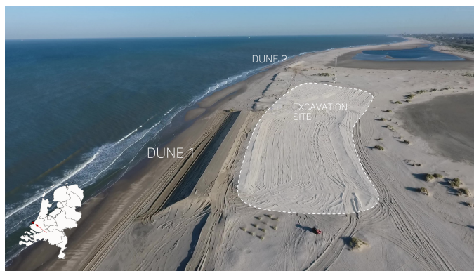
Figure 3.2. Aerial view of the field site including Dune 1, Dune 2, and the excavation site from which sediment was excavated for the construction of both dunes. The field site location within the Netherlands is displayed on the inset map.
