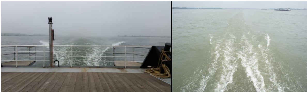
Figure 2: Comparison of wave profile on the 55 meter supply vessel without Hull Vane (left) and with Hull Vane (right) at 13 knots, as seen from the aft deck during sea trials (Uithof, Moerke, Van Oossanen, Van Oossanen, & Zaaijer, 2014)
