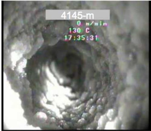
**Figure 1-3 NaCl scale in the perforated zone of a gas well before fresh water treatment <sup>[a]</sup>**
