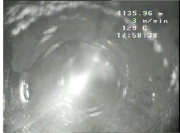
**Figure 1-4 Perforated zone after fresh water treatment <sup>[a]</sup>**
