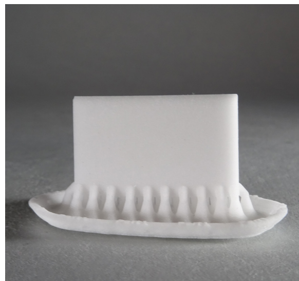
Figure 3.5-1 Wire like structure supporting a solid object.
