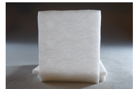
Figure 3.6-9 Cracks throughout the surface after firing
