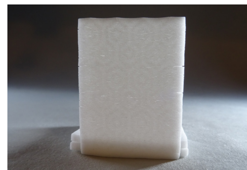
Figure 3.6-16 When internal structure is too small it will not translate clearly
