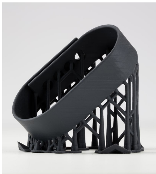
Figure 2.3-3 Formlabs support structure
