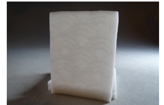
Figure 3.6-10 Cracks throughout the surface after firing
