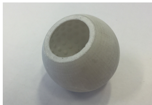
Figure 3.6-11 Green state hollow sphere with internal structure
