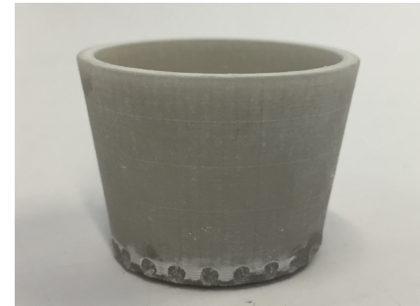
Figure 3.6-6 Green state controlled cracking sample
