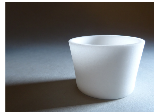
Figure 3.6-7 No cracks occurred during firing
