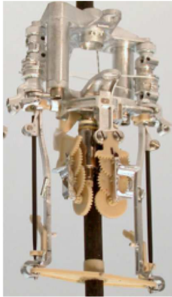
Figure 4-8: Assembled control system as found in the Nano Hummingbird. Adapted from Keennon, Klingebiel, Won, & Andriukov (2012).
