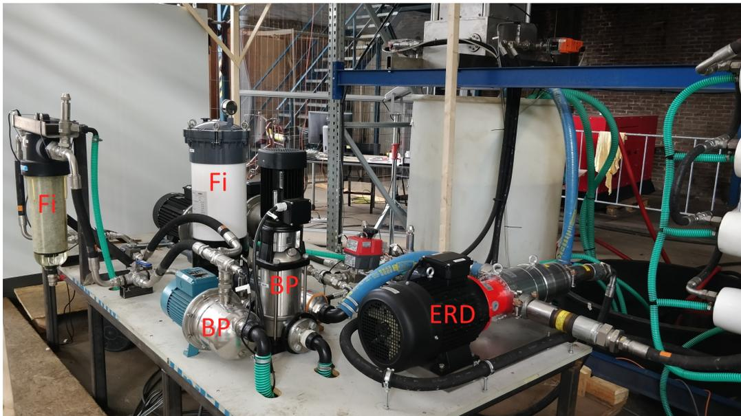
Figure C.3: A close up of the setup, clearly showing the filters, boost pumps and ERD
