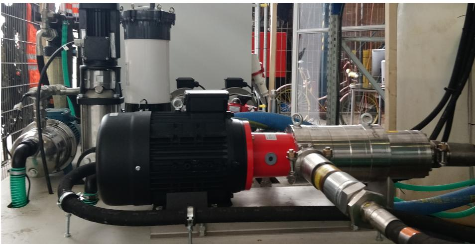
Figure 5.3: The iSave ERD as it is installed in the MicRODOT test setup.
