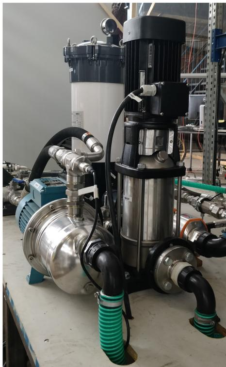
Figure 5.5: The setup has two boost pumps. The left boost pump is the large pump, feeding the ERD. The right pump feeds the High Pressure pump.
