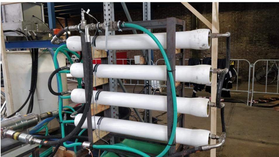
Figure 5.4: The RO setup, showing 4 membranes installed in pressure vessel in a parallel configuration.
