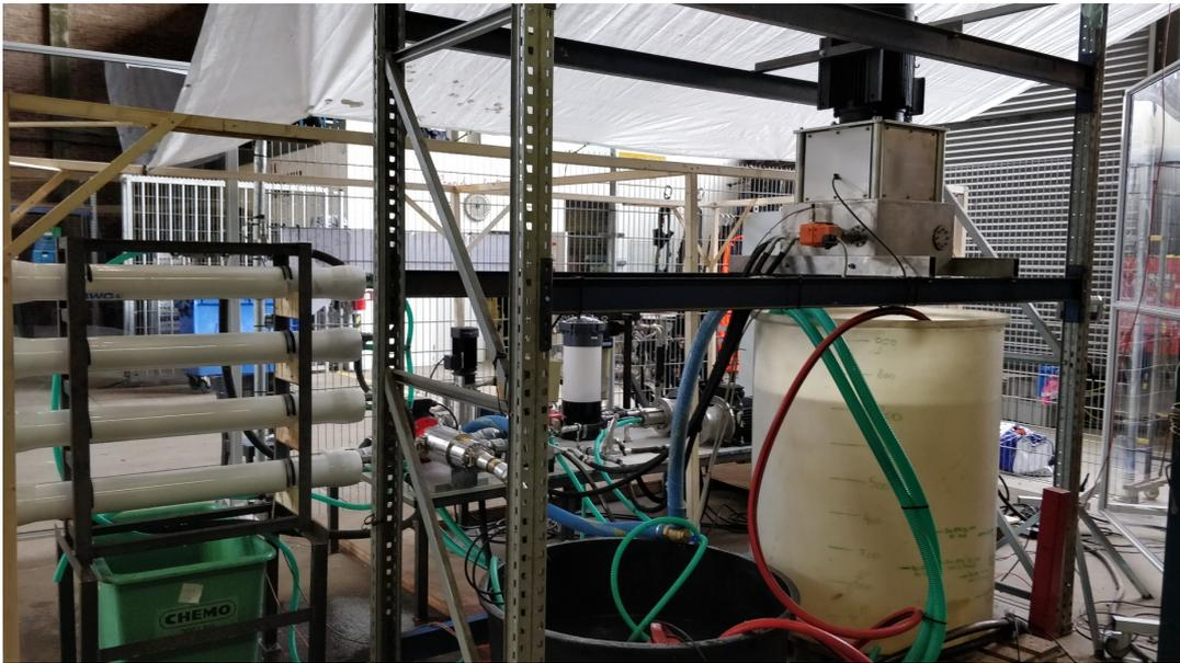
Figure C.2: The three water tanks shown in the figure are the permeate tank (green, left), the concentrate tank (black, middle) and the feed water tank (white, right).
