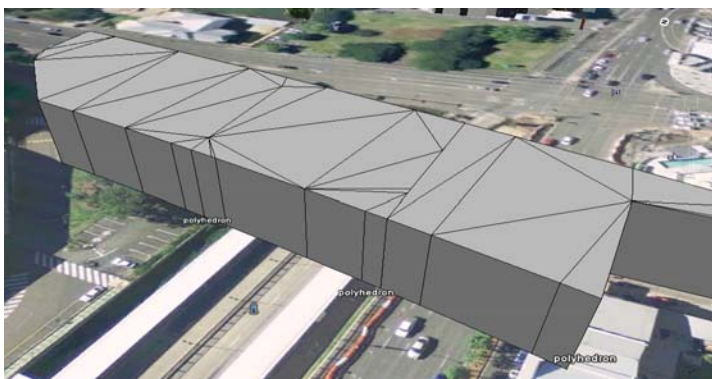
Figure 18. Sections of a tunnel parcel. The top surface is not horizontal, and has been triangulated. The sides are vertical and are composed of rectangles. (The z values have all been increased by 40m so that it is visible above ground)
