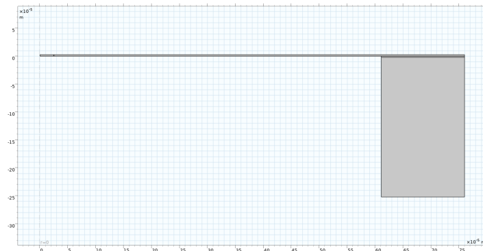
Figure 6.1: 2D drawing for modelling of membrane-based opto-mechanical AE sensors within a 2D axisymmetric component.
