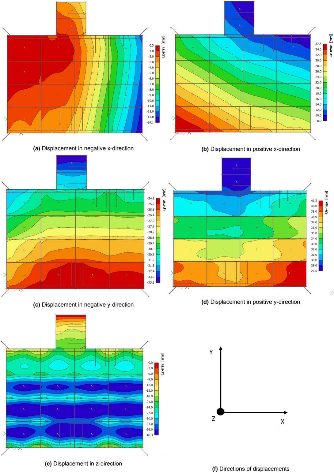
Figure 4.19: Extreme displacement of reusable jetty deck
