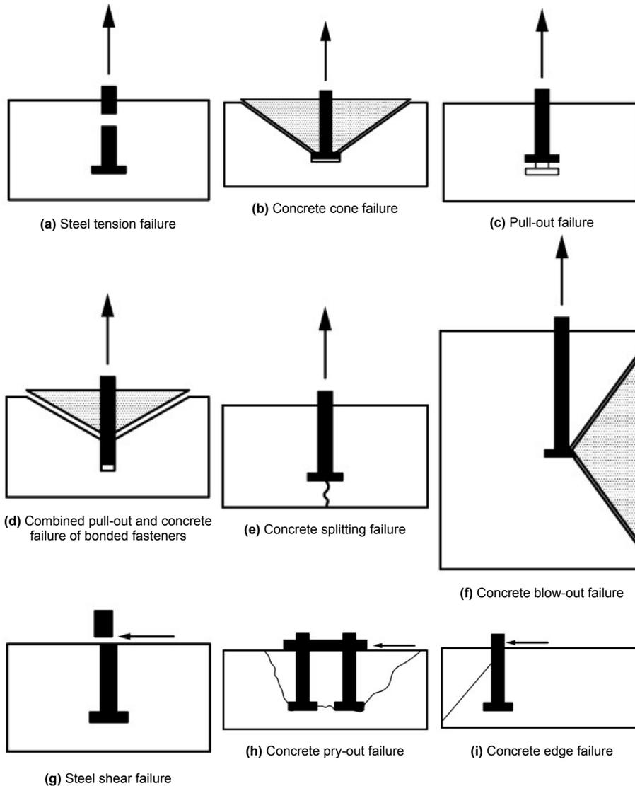
Figure 5.4: Failure mechanisms of anchor bolt [49]
