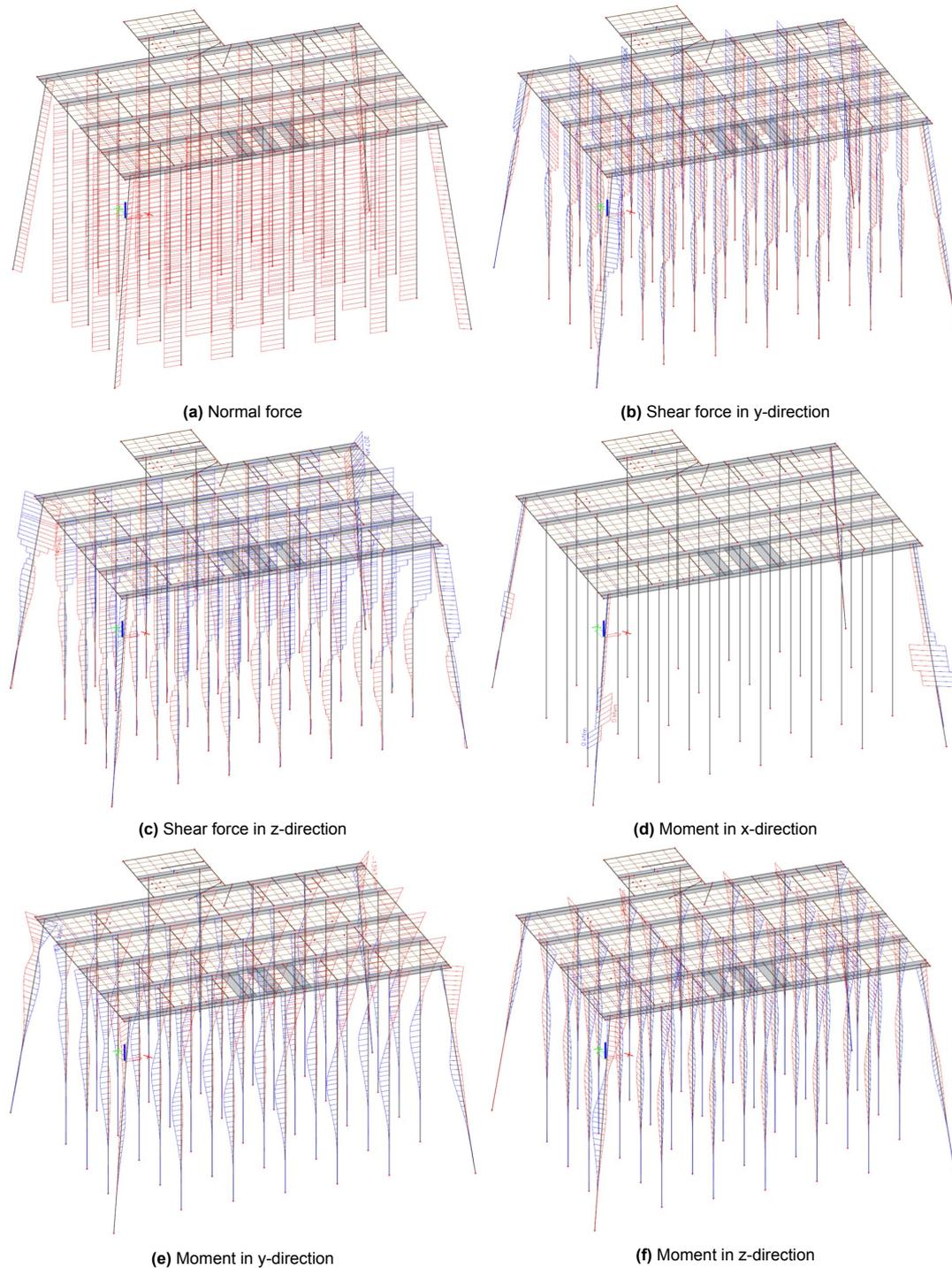
**Figure 3.5:** Internal forces in piles of reference jetty
