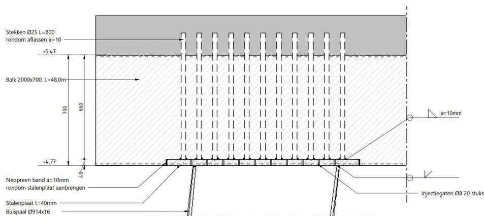
**Figure C.3:** Detail of fixed pile to beam connection [61]
