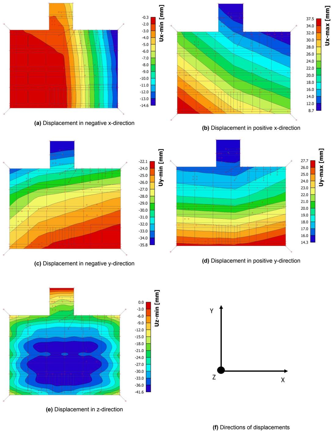
Figure 3.8: Extreme displacement of reference jetty deck
