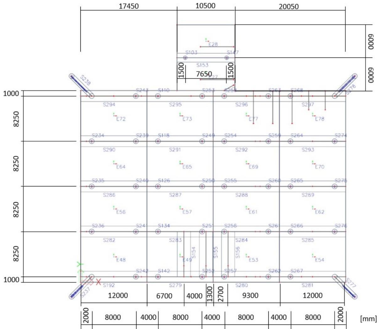
**Figure D.5:** Layout of reference jetty model
