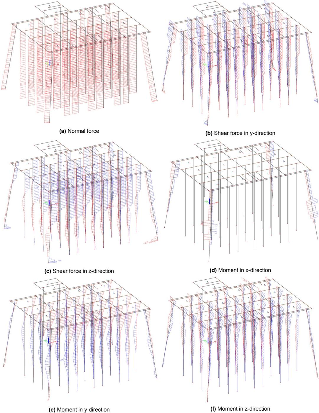
Figure 4.8: Internal forces in piles of reusable jetty
