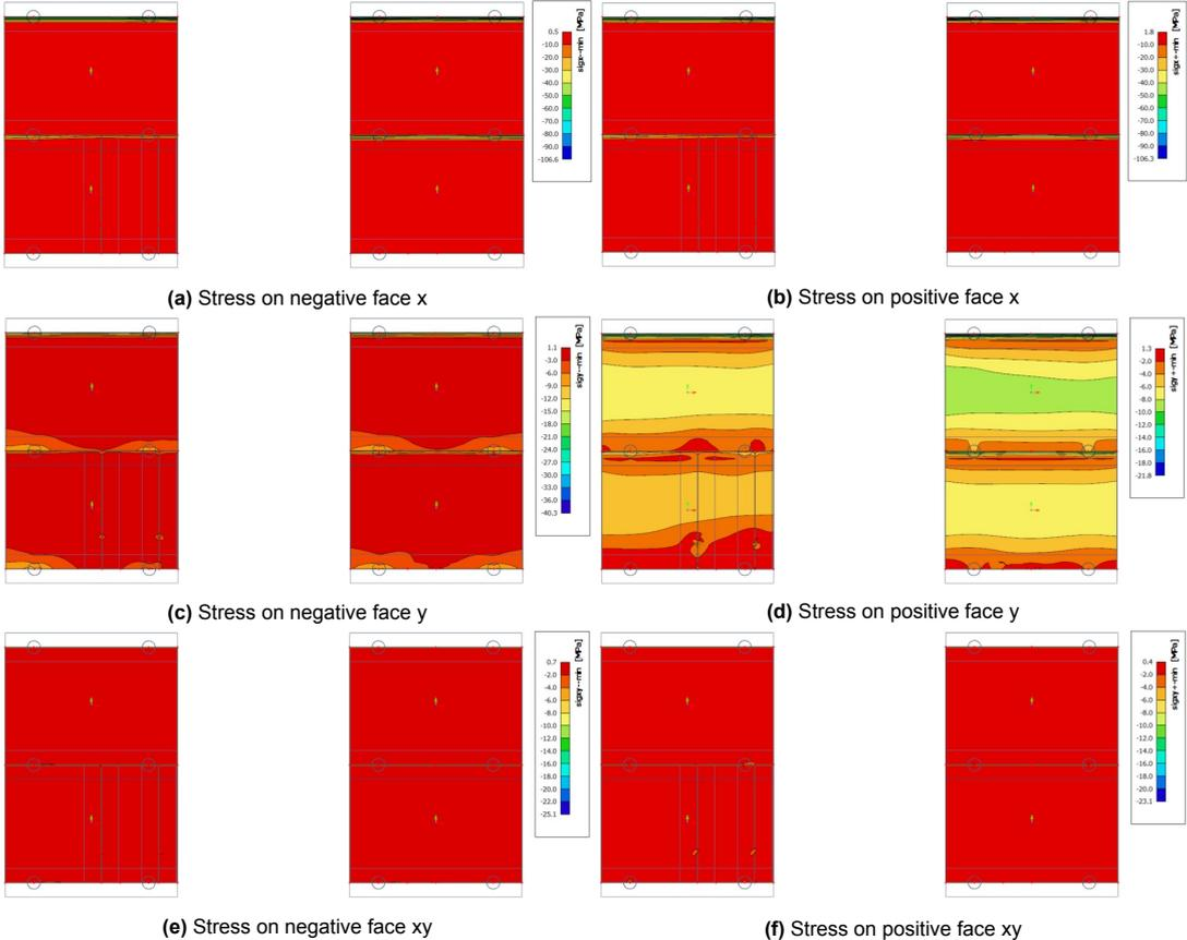
Figure F.10: Extreme negative stresses in faces of modules
