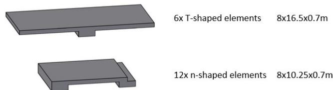
Figure E.10: All prefab elements used in variant 2
