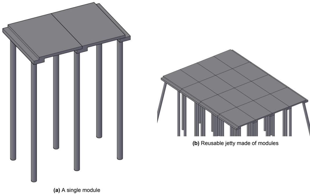
**Figure 6.1:** Layout of modular reusable jetty structure
