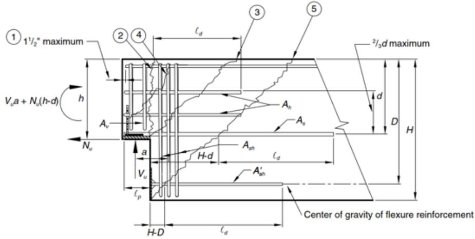
Figure 5.2: Reinforcement and crack formation in a dapped end connection [29]
