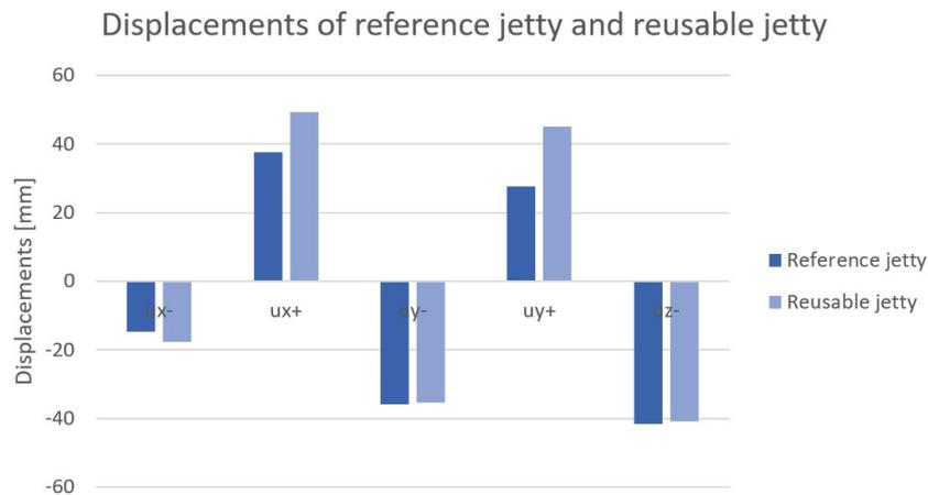
**Figure 4.14:** Extreme displacements of reference jetty and reusable jetty
