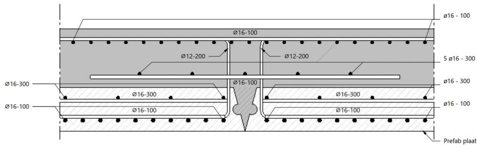
Figure C.5: Details of deck plate edges [61]
