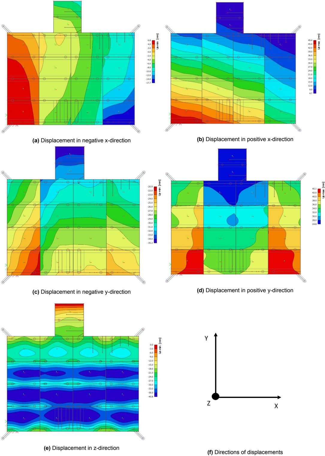
Figure 4.13: Extreme displacement of reusable jetty deck
