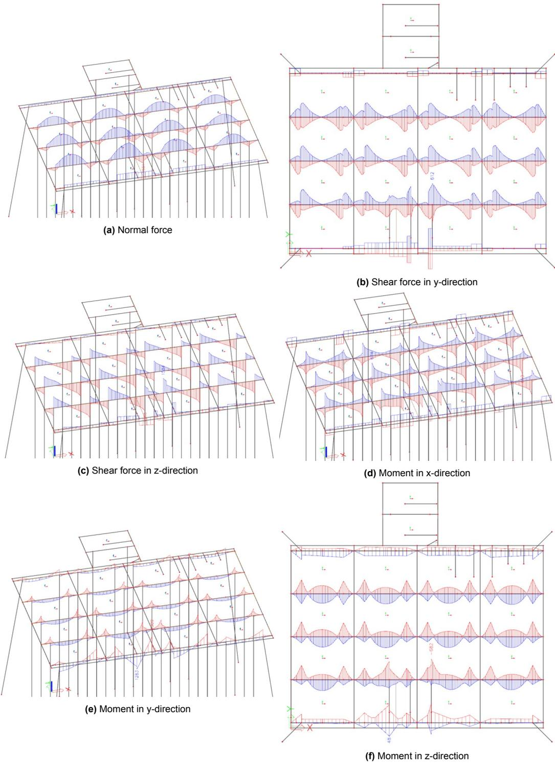
Figure 4.6: Internal forces in rib plates of reusable jetty
