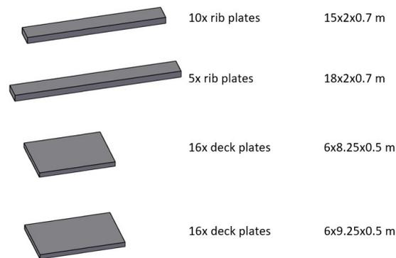
Figure E.2: All prefab elements used in variant 1
