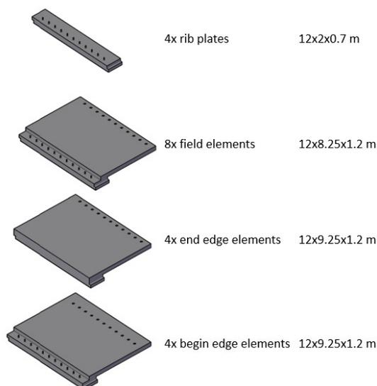
**Figure 4.3:** All prefab elements used in variant 3
