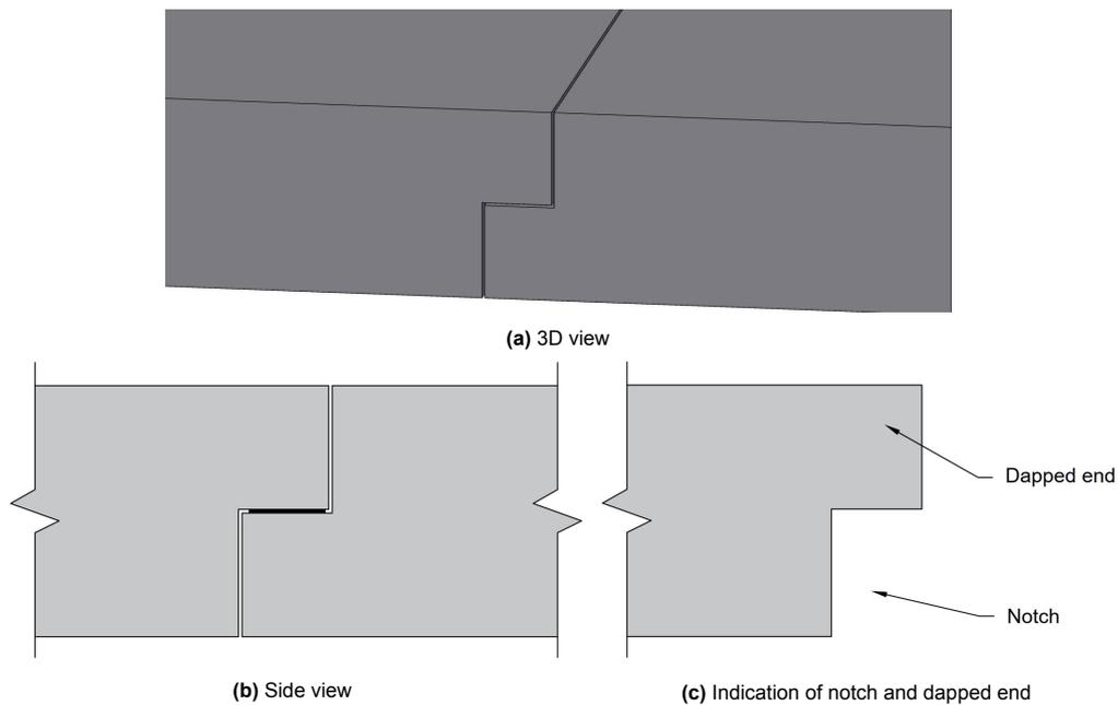
**Figure 5.1:** Shear rib plate to rib plate connection
