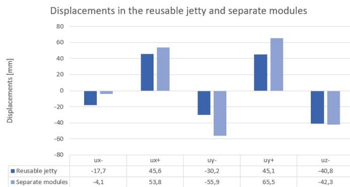
**Figure 6.3:** Comparison of displacements in reusable jetty and separate modules
