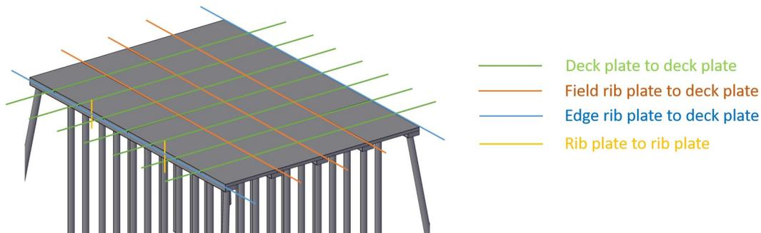
**Figure E.3:** Connection types in variant 1
