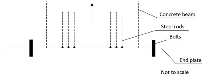
Figure E.26: Failure mode 1: Yielding of rods
