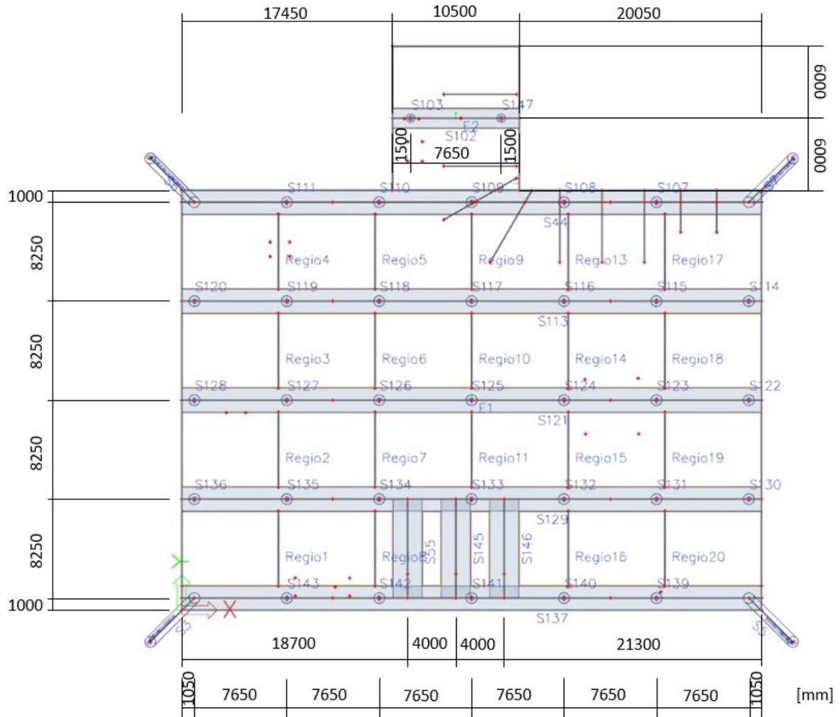
Figure D.4: Layout of reference jetty model
