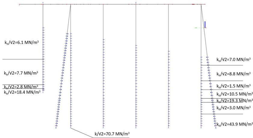
Figure 3.1: Soil modelled as springs in SCIA Engineer
