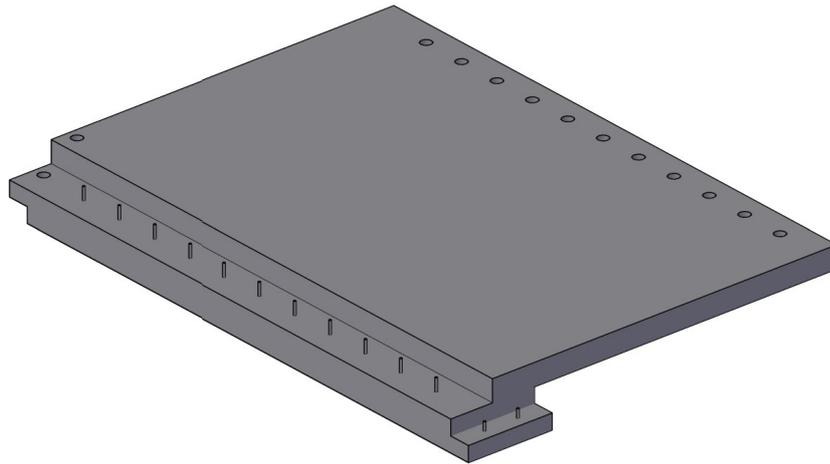
**Figure 4.17:** Example of anchor bolts in shear connection
