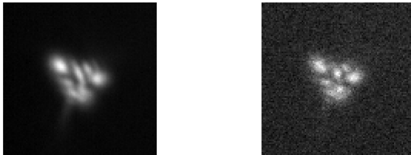
Figure 6-1: Images of the same out-of-focus aberrated bead. (Left) Image resulted as the average of 69 images of the same bead subject to the same aberrations. (Right) Single image as recorded by the sensor.
