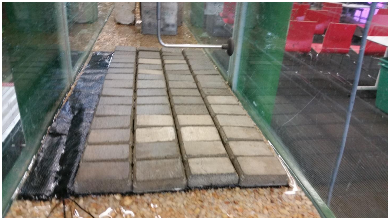
Figure 4.2 The open-end edge of the block mat
