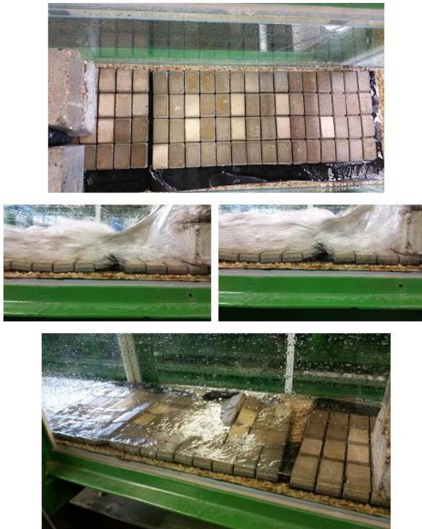
Figure 5.18 Frame to frame failure of the block mat (transition with gap)
