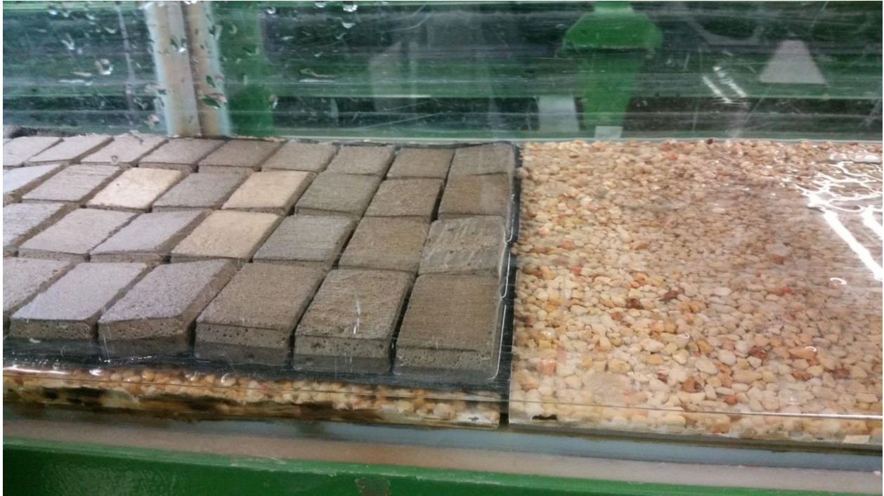
Figure 4.3 'Fixed' edge by placing the geotextile of the mat under the artificial bed
