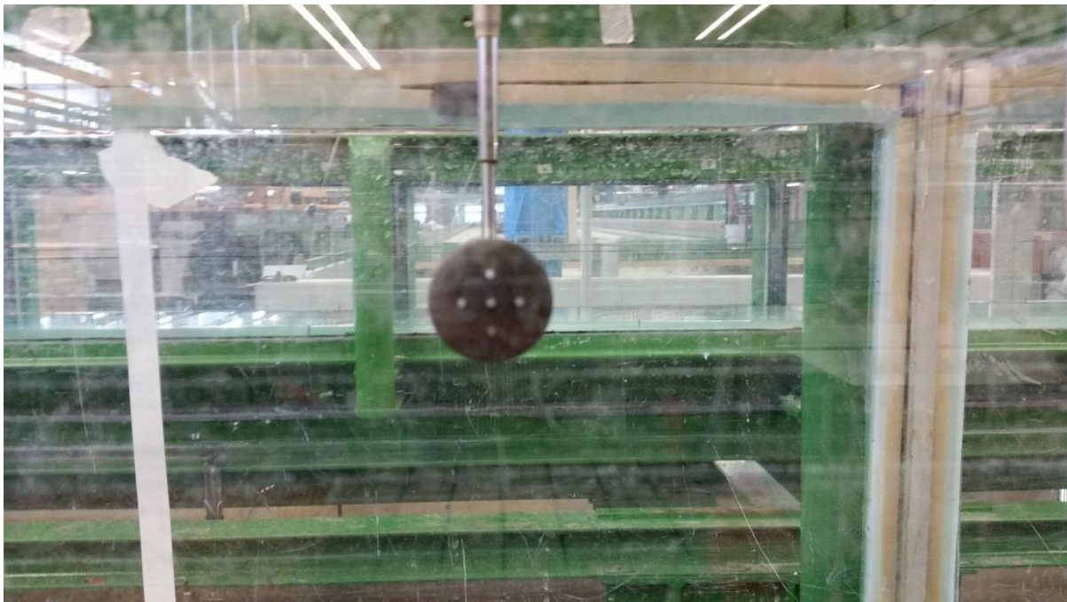
Figure 4.4 Electromagnetic Flow meter (EMS)
