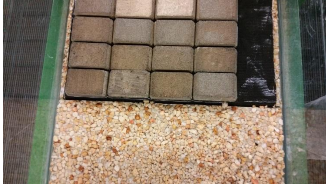
Figure 5.3 'Fixed' upstream edge of the block mat
