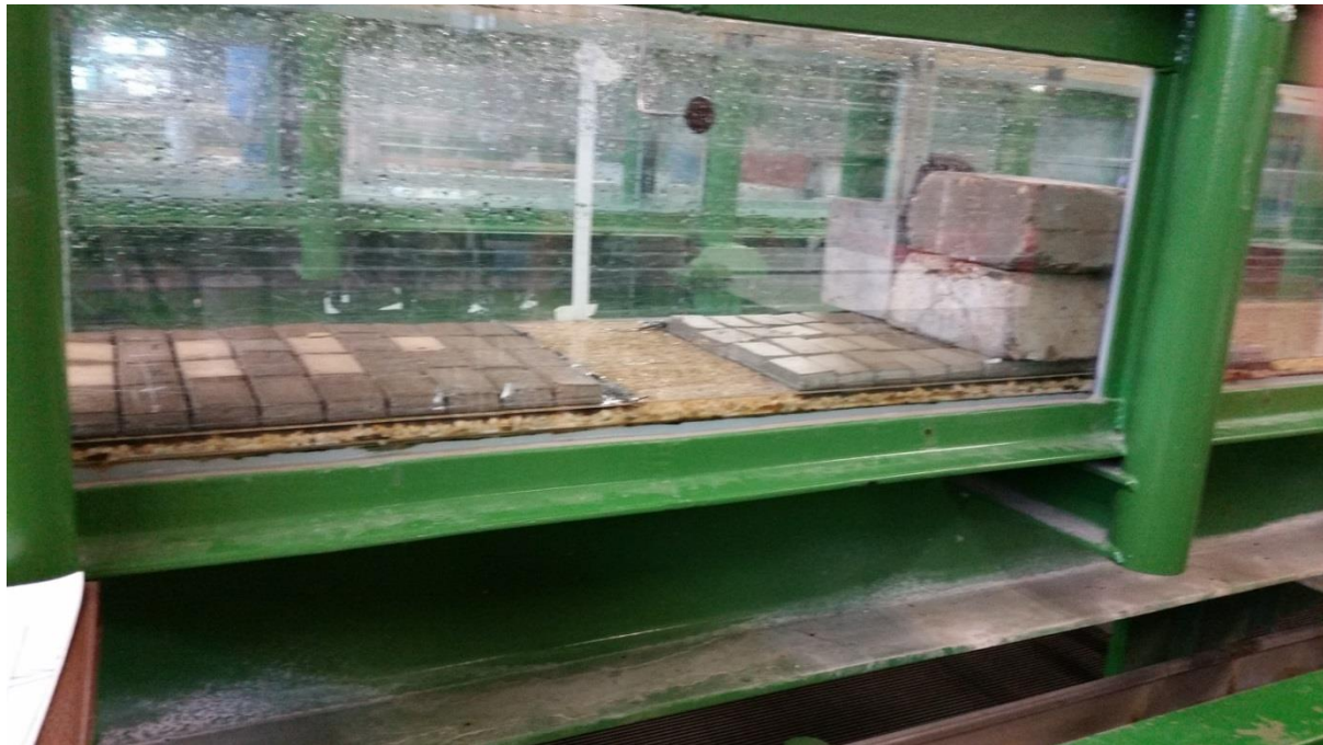
Figure 4.1 Test on a ‘free’ to move block mat
