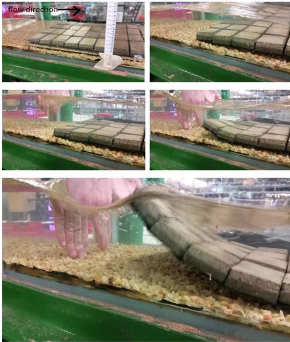
Figure 5.2 Frame to frame failure of the block mat (hands upstream)
