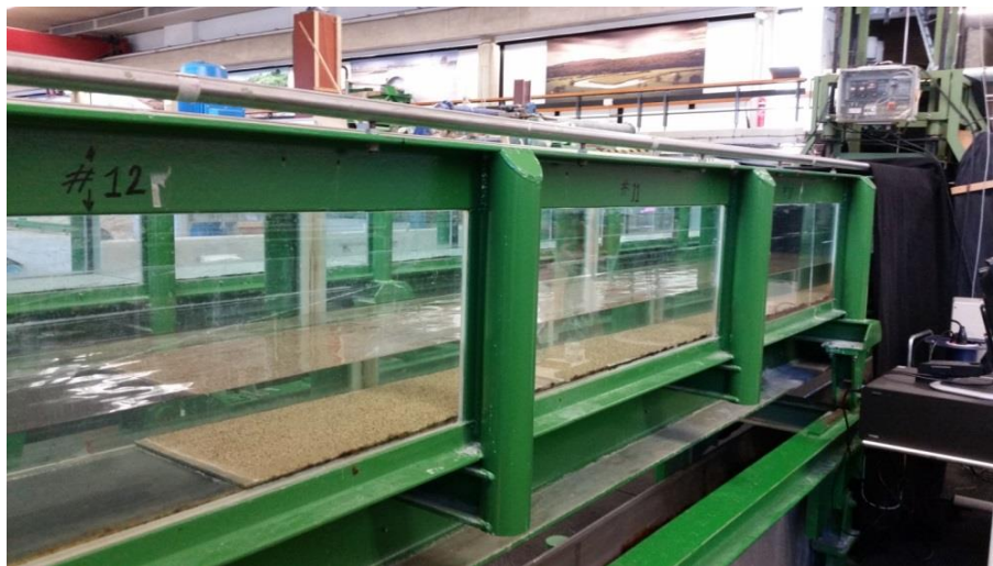
Figure 3.3 Water flume for experiments under current loads
