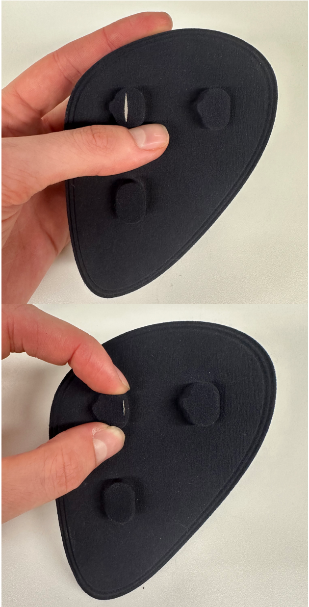
Figure 13.1.2: Anisotropic fragility of the MJF printed base plates.
