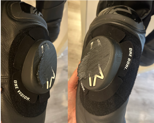
Figure 13.1.1: Kneeslider with molten TPU which has been transferred away from the friction surface as a result of high friction heat.
