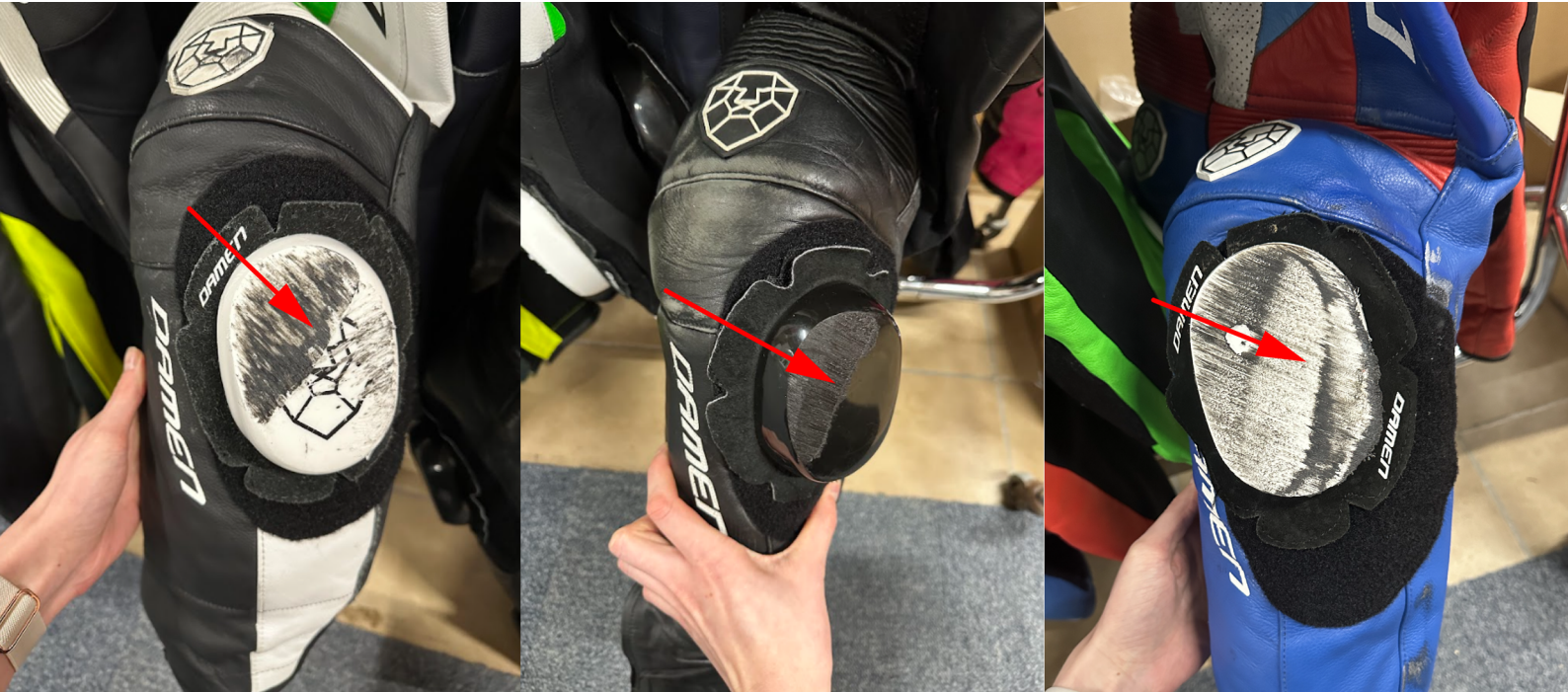
Figure 16.4.3: Universal shear force direction on sliders during cornering.
