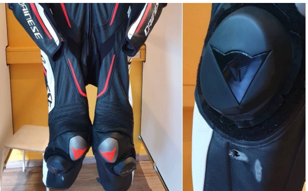
Figure 10.1.2: Ill-fitting standard size suit resulting in contact point aberrancy (suit protection does not align with joints in body and therefore the suit does not accurately represent where the rider touches the tarmac) (De Zilveren Naald, 2021).
