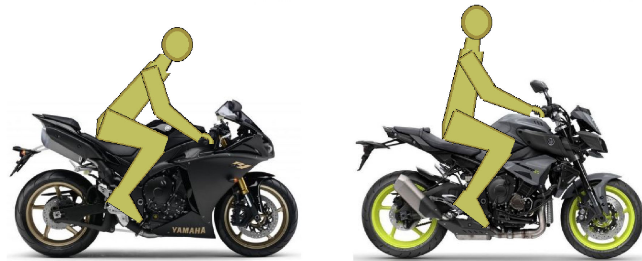
Figure 2.1.2: Sports bike (left) vs Naked bike (right) (cycle-ergo, 2024). 2012 Yamaha R1 Calculated seat height: 833 mm Forward lean: 39° Knee angle: 72° (smaller number means more bent) Hip angle: 58° (smaller number means more crouched) 2019 Yamaha MT-10 Calculated seat height: 828 mm Forward lean: 11° Knee angle: 75° (smaller number means more bent) Hip angle: 84° (smaller number means more crouched)
