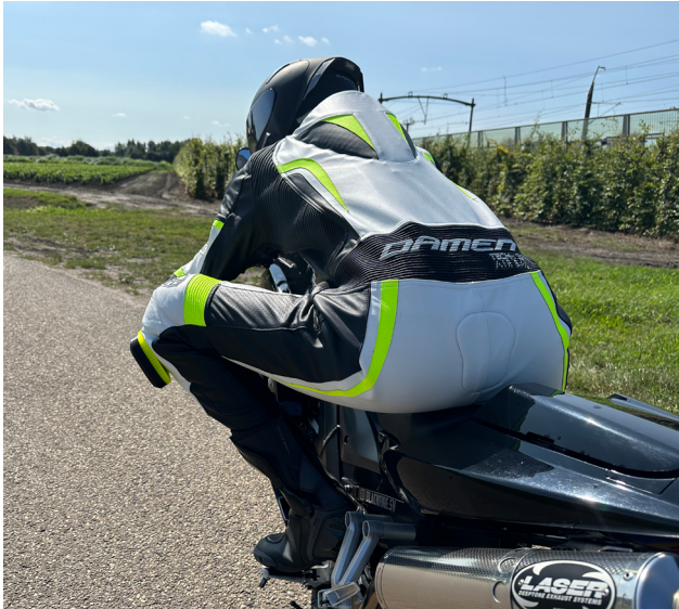
Figure 16.3.1: First user test shows new design aspects which call for attention and improvement as a gap shows up between slider and leather.
