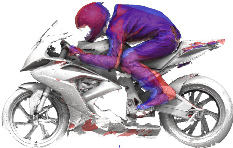
Figure 10.2.2: Comparison of body positioning on a motorcycle as a result of body proportions (Blue: P1, Red: P3).
