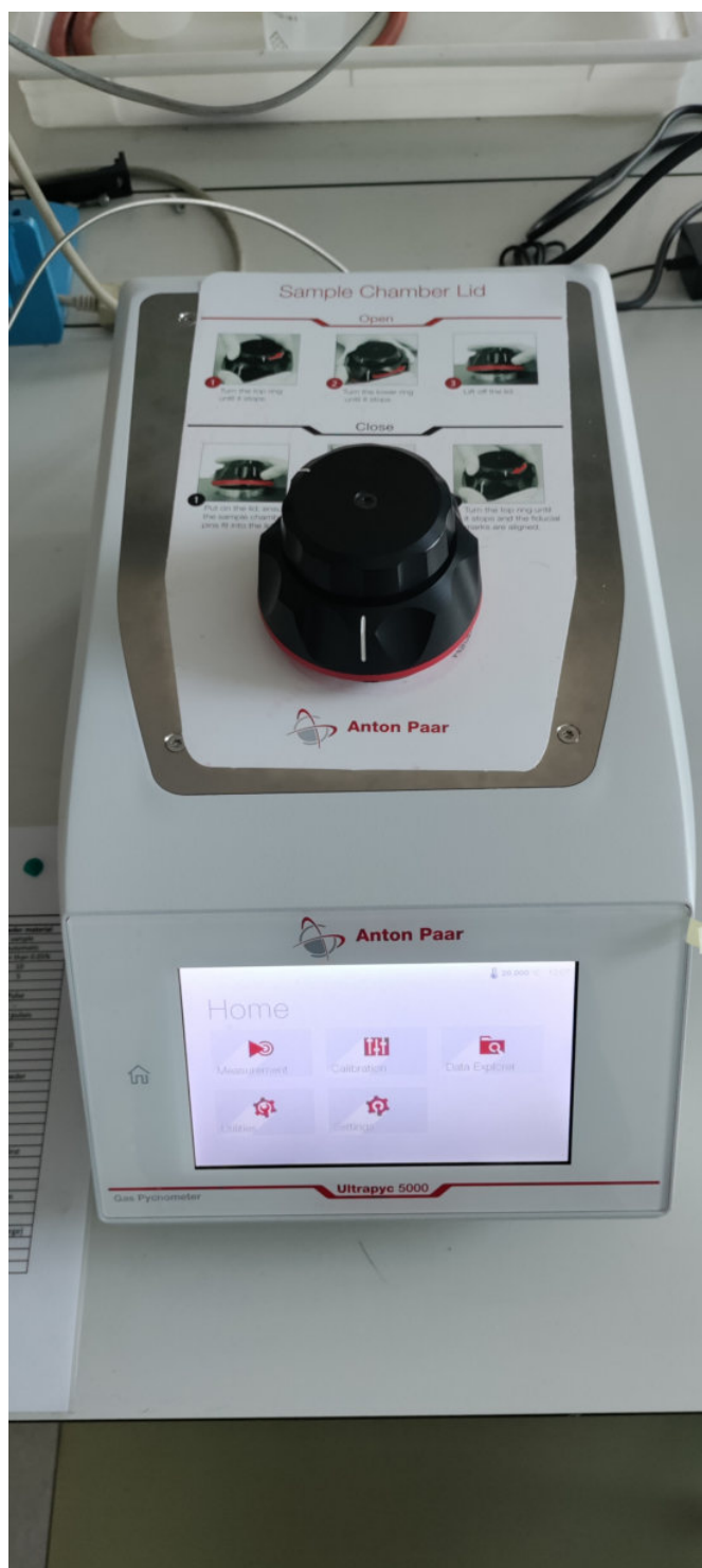
Figure G.33: Helium pycnometer used to measure the volume and density of the dried samples before testing
