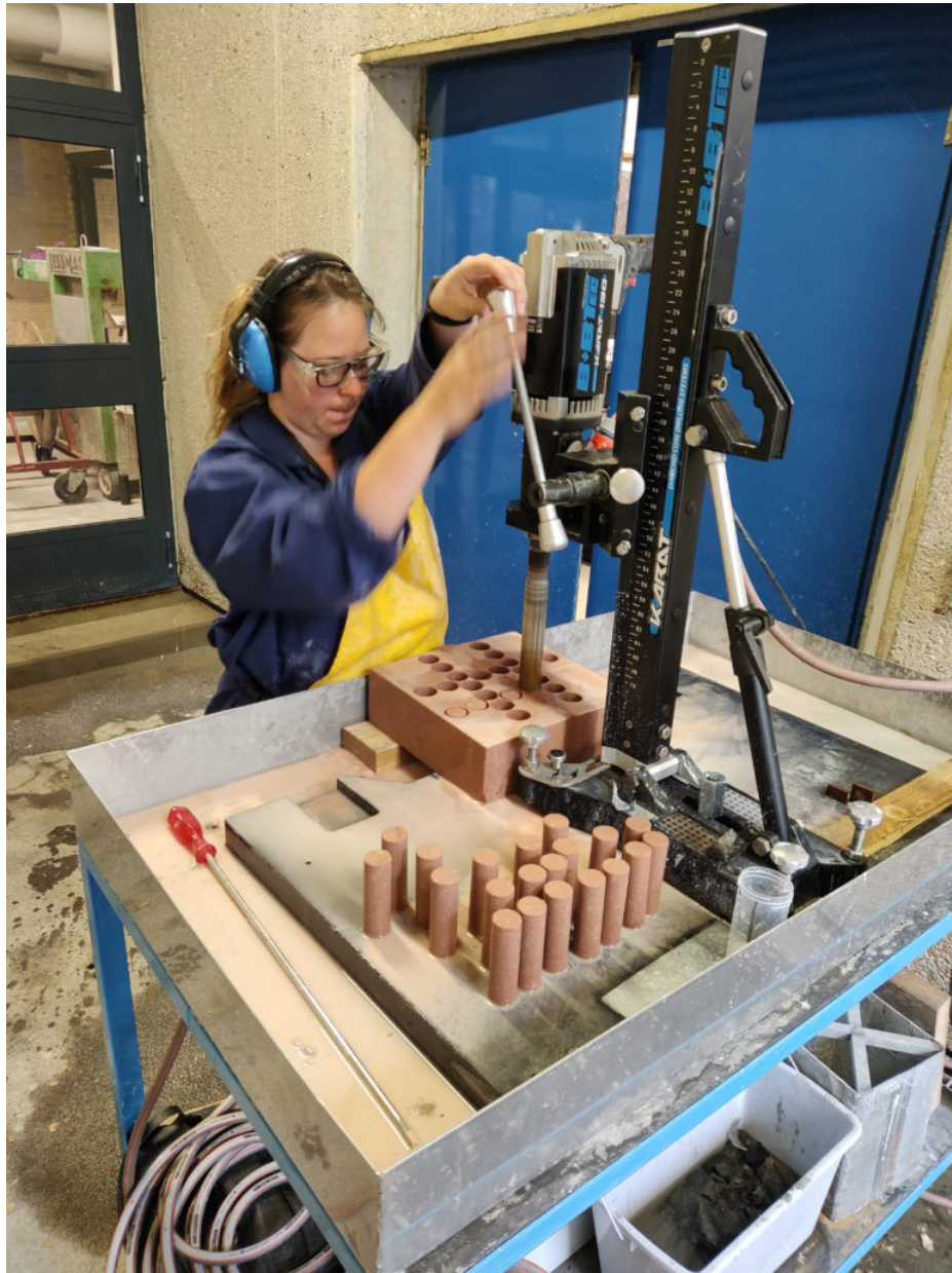
Figure G.30: Coring machine. Cores being made to the Red Felser sandstone block from Germany
