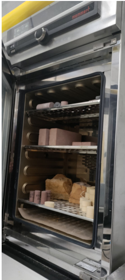
Figure G.32: Oven used to dry the samples. Temperature = 60°C
