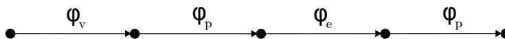
Figure 4.3: A chain of base operators defines the operator to add a link \varphi_l , each vertex in this chain represents an in-between mechanism representation.
