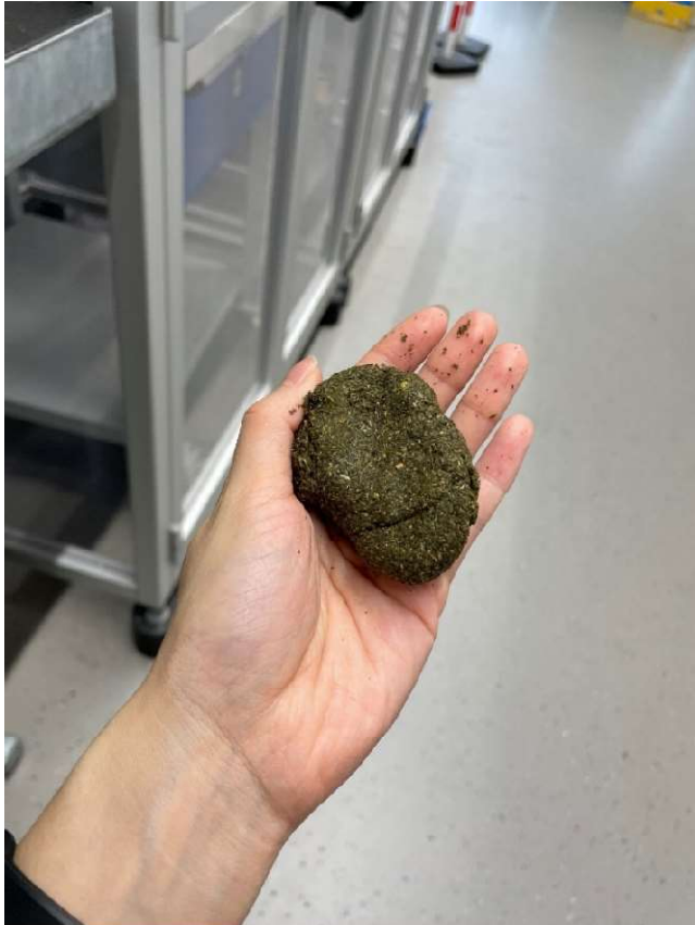
figure 57: The next day, which is 17 hours later, the material was still mouldable
