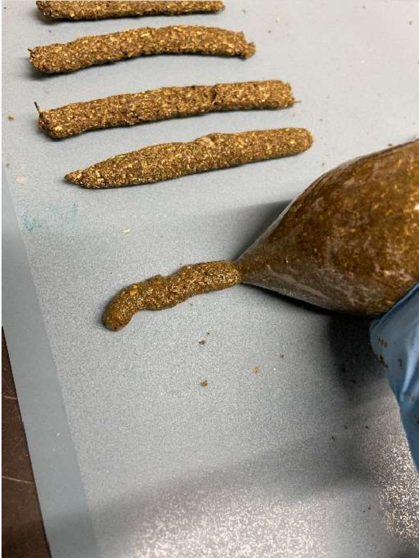
figure 50: The material was extrudable. It could not be moulded by hand because it stuck to the gloves.
