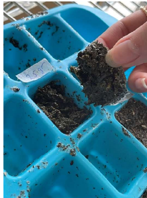
figure 40: Demoulding the samples too early can cause the samples to break
