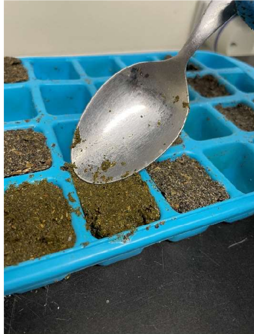
figure 49: Moulding the material was possible using spoons and pressing it in the mould
