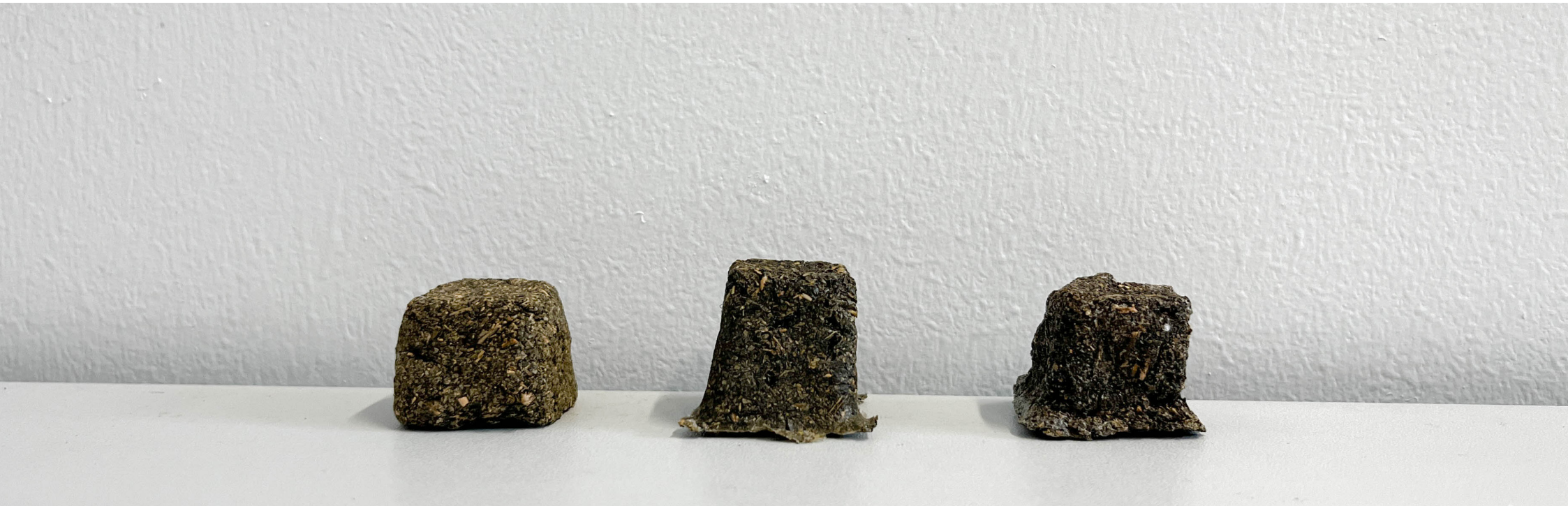
Figure 5.13: shrinkage occurs in flat surface that go towards the middle of the sample, as can be seen in the sample on the right.
