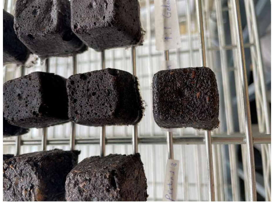
figure 28: Gelatine samples that were demoulded earlier have a glossy finish, and freshly demoulded gelatine samples look like cake.
