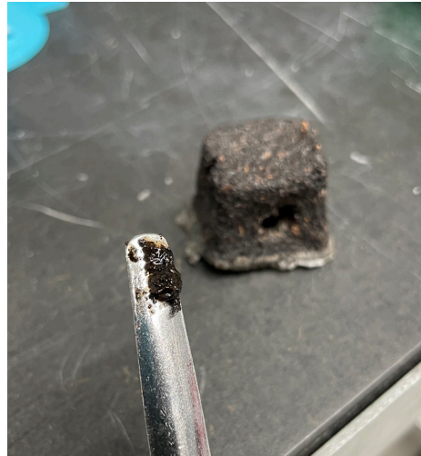
Figure 5.16: Inside of the material is liquid while the outside is hard
