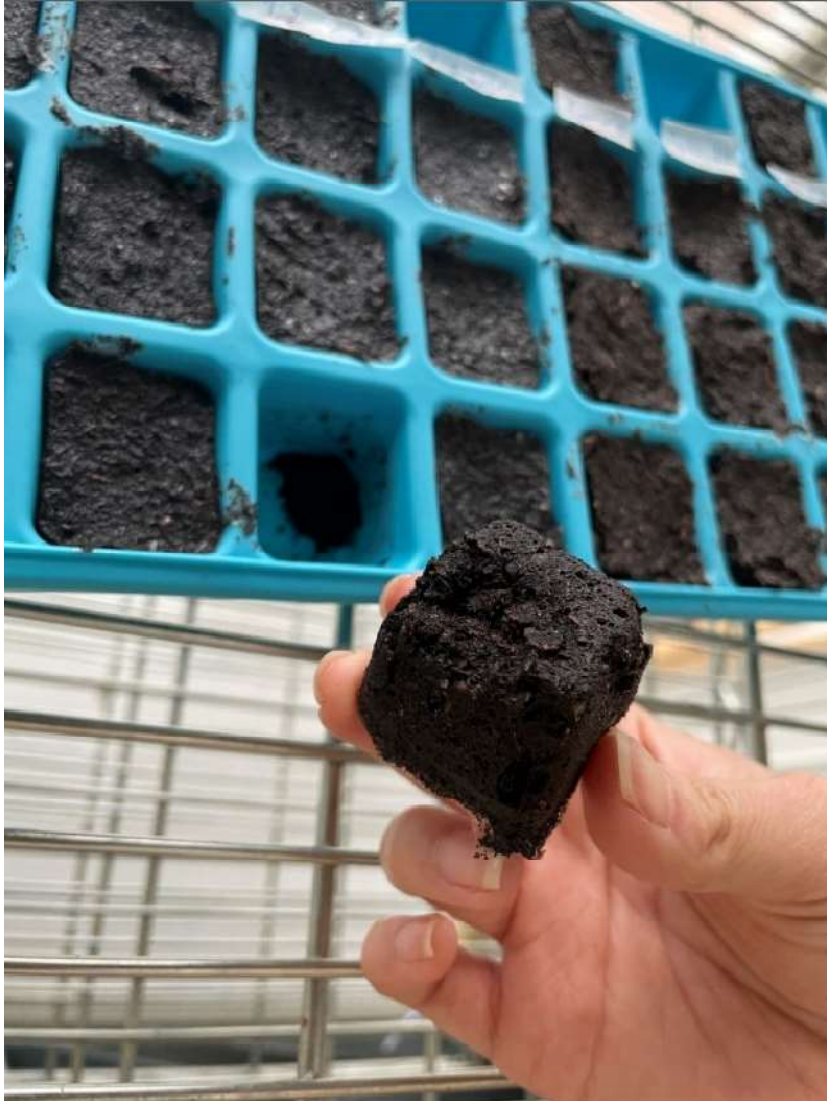
figure 27: Gelatine samples and agar agar could break when trying to demould too early
