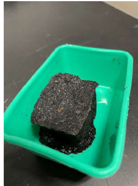
figure 38: Gelatine 1:3 starting to lose its shape after some force was pressed on it.
