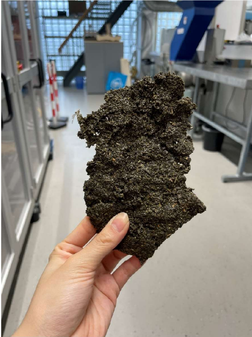
figure 54: Gelatine with 60 ml water solidified fast.
