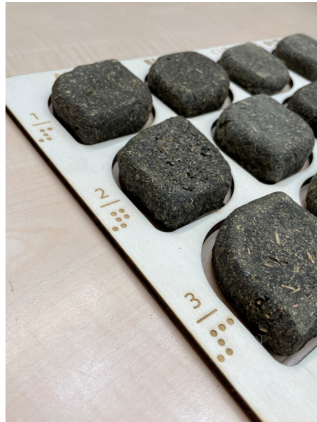
Figure 8.21: Laser engraved tactile patterns.
