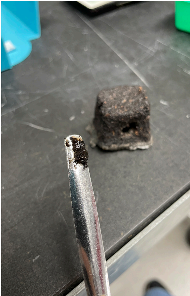
Figure 5.4: when the gelatine sample was heated, the outside remained solid, but the inside was liquid
