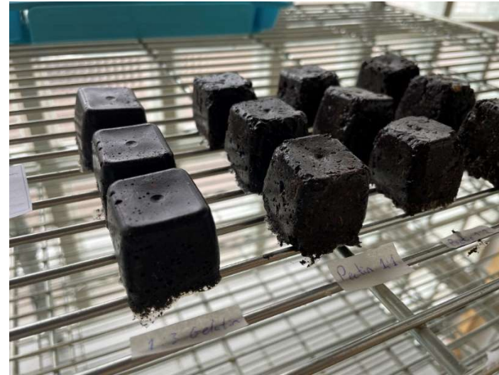
figure 25: Gelatine has a very different surface finish compared to pectin
