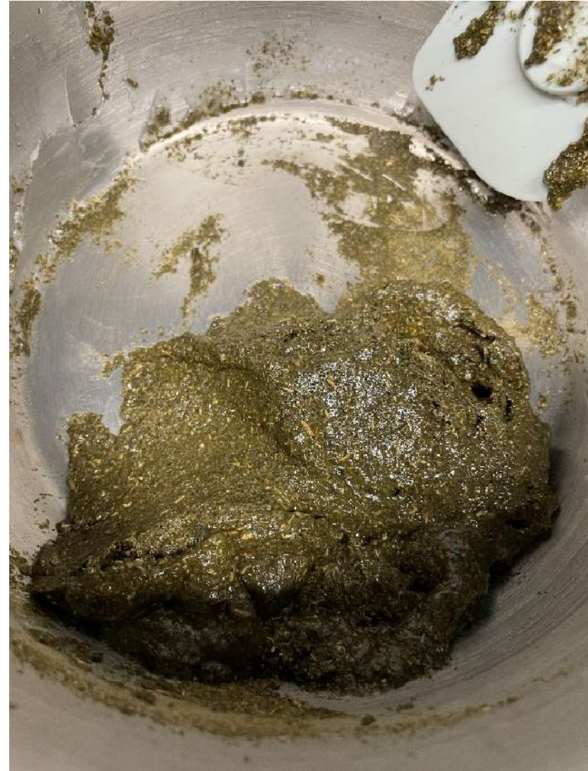
figure 47: The binder with the tea resulted in a paste
