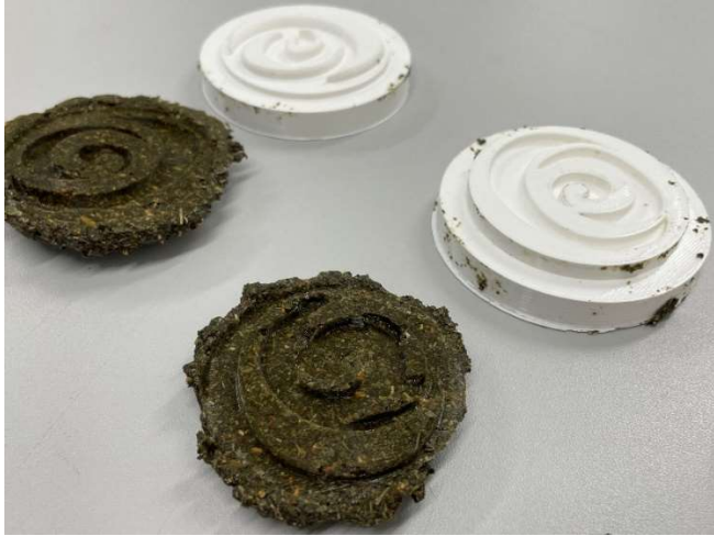
figure 66: some details were not conveyed, especially if the mould had small gaps.
