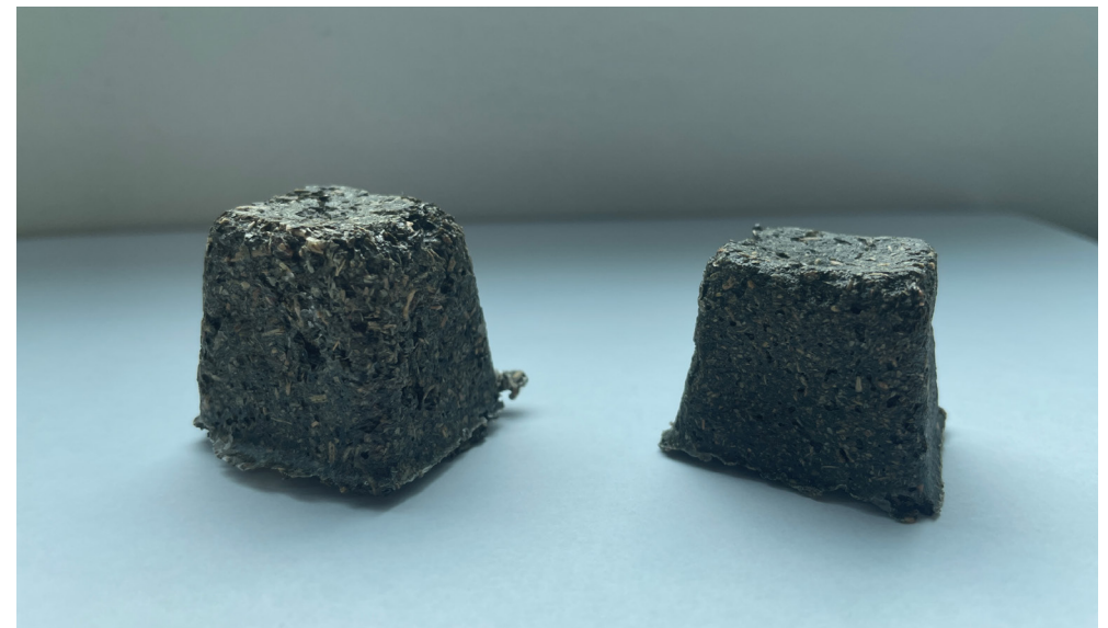
Figure 5.15: left: 53% water, right: 57% water. The 57% water sample is more homogenous.
