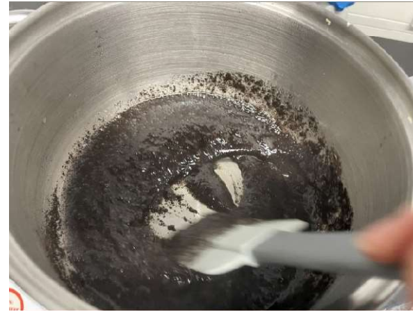
figure 3: Gelatine 1:1, 70 degrees, turning more solid
