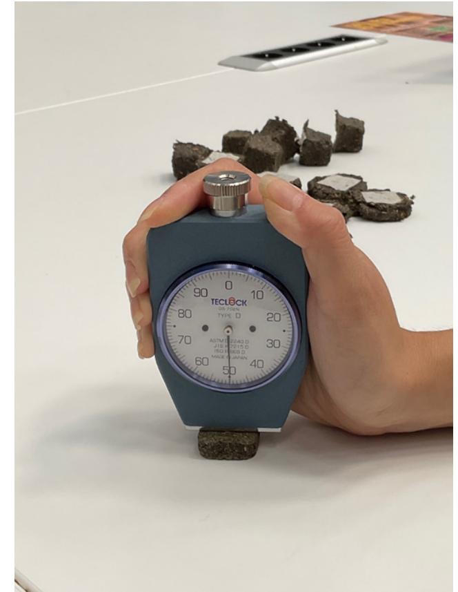
Figure 6.9: using a durometer to measure the hardness.
