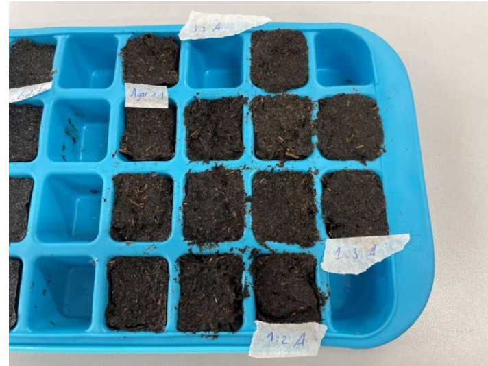
figure 22: The samples drying in their moulds
