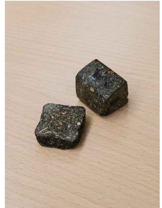
Figure 5.26: Sanded material and coated with TruOil
