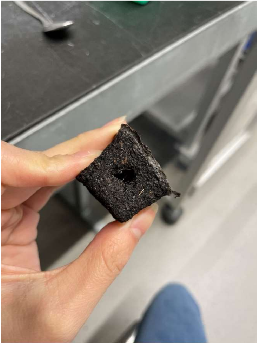
figure 35: Holes could be poked, outer membrane is hard but inside not
