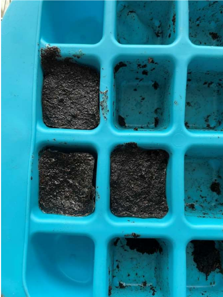
figure 29: Shrinkage of gelatine samples
