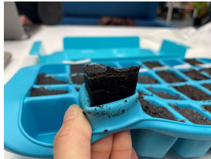
figure 23: the top dries first. The silicone enables ease of demoulding.
