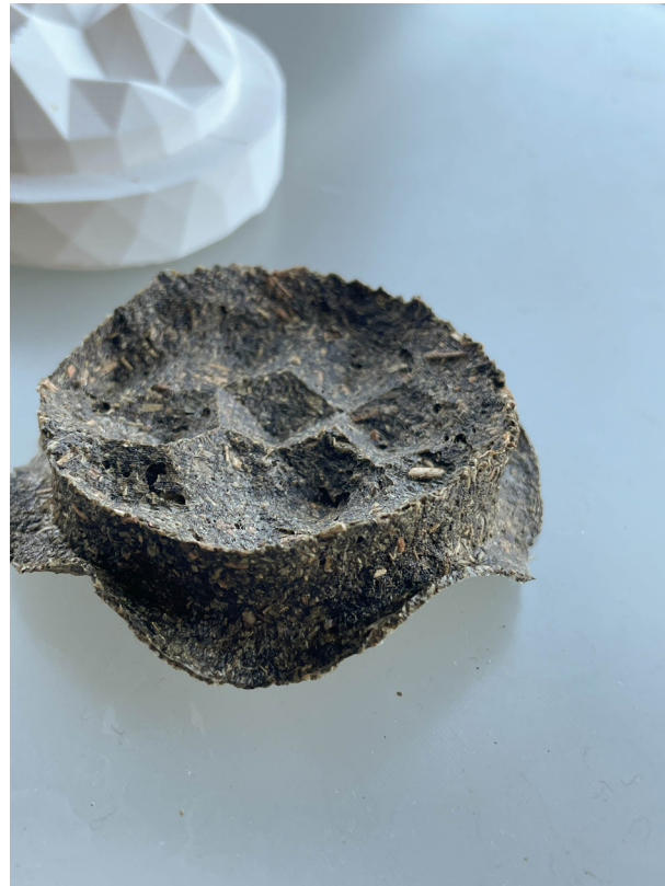
Figure 5.25: when dried, the thin material warps severely.
