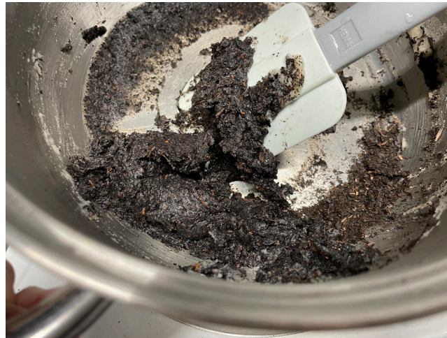
Figure 5.9: a low processable material, as it cannot be stirred and needs hands to knead and mould.
