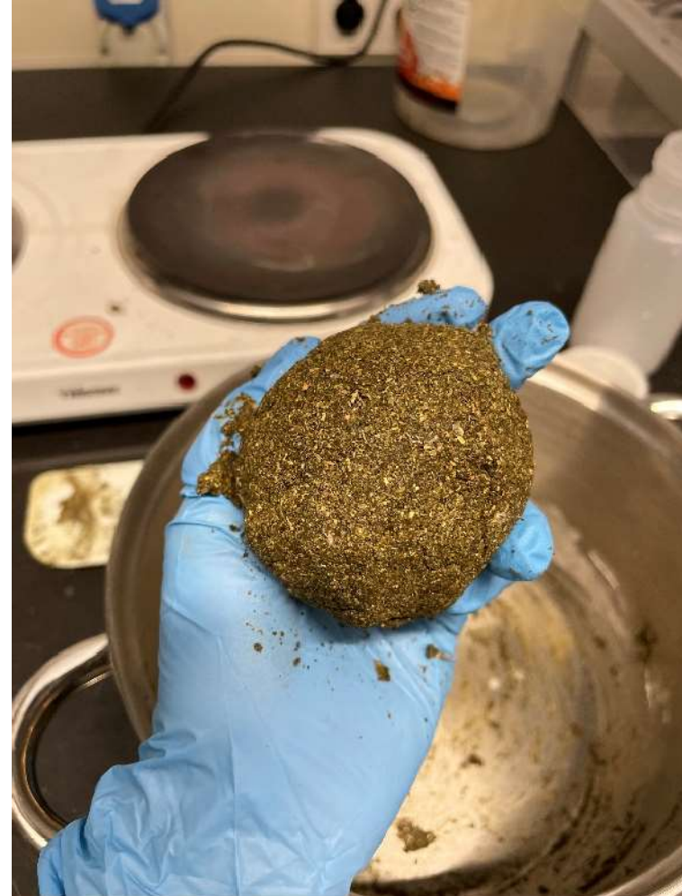
figure 42: The material resembles clay and can be moulded by hand.
