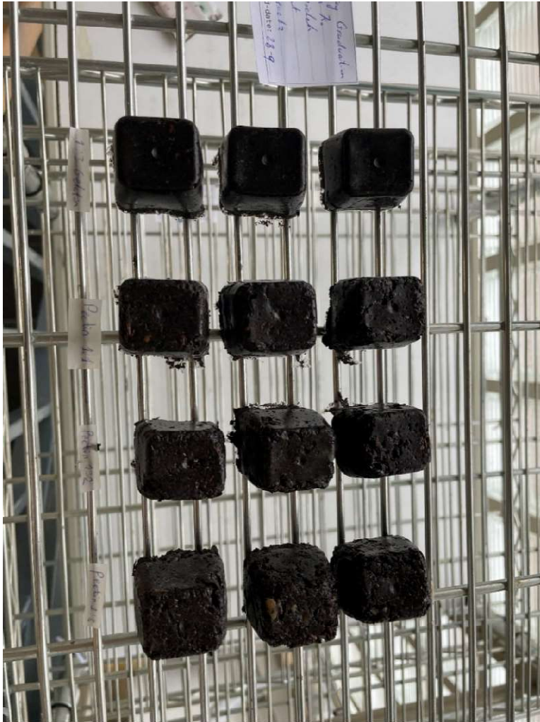
figure 24: The samples that could be demoulded the same day, plus the two gelatines ( a bit later)
