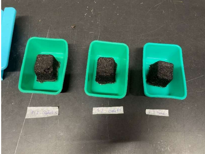
figure 32: The samples in a different mould to be melted
