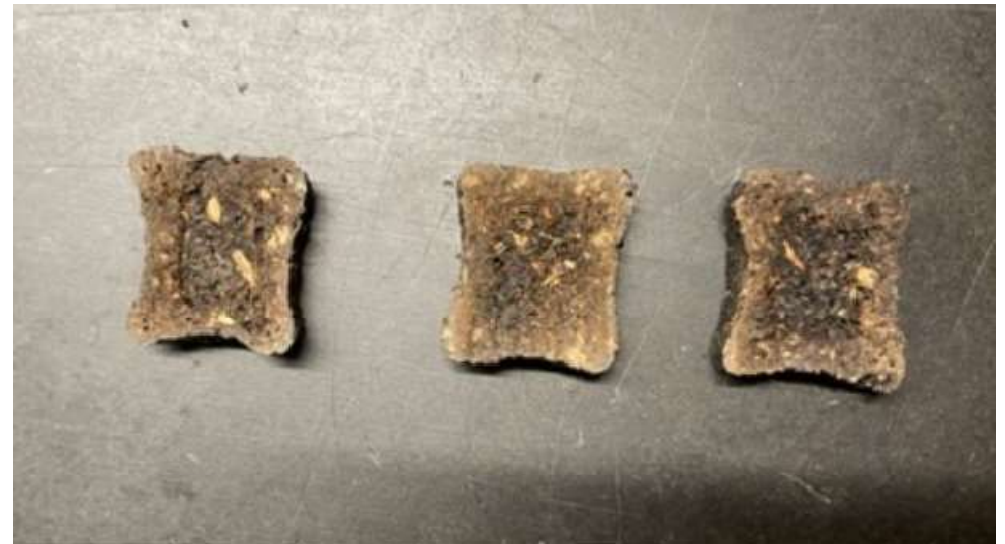
figure 31: samples sawed in slabs turned out to be not completely dried inside.
