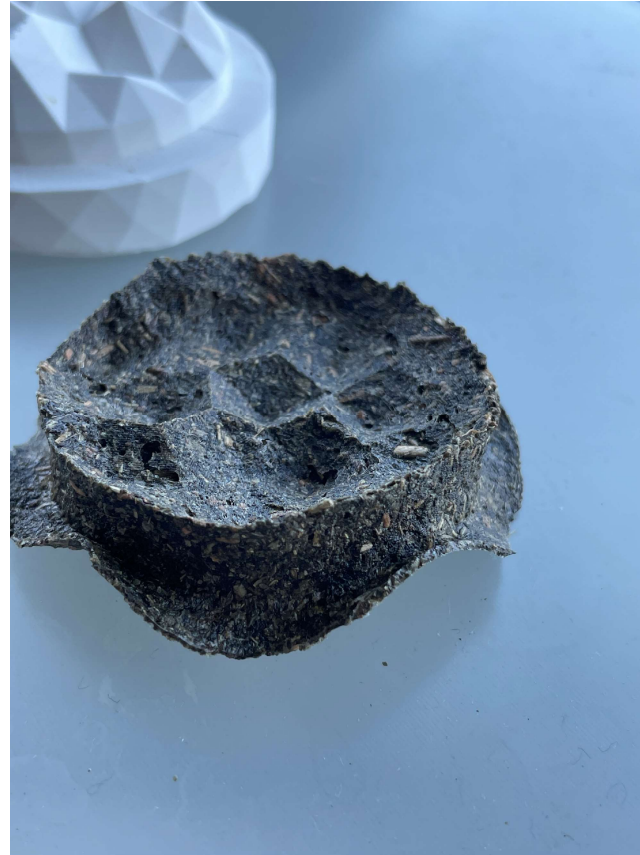
figure 70: the thin material warps when dried.
