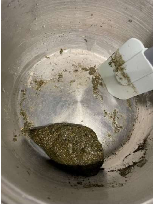
figure 55: beeswax causes the material to not stick to the pan
