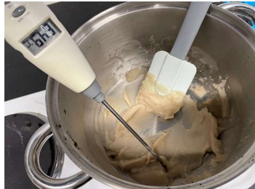
figure 17: Agar agar 1:3 at 65 degrees is like a paste
