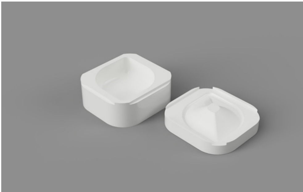
Figure 8.18: A 2 sided mould
