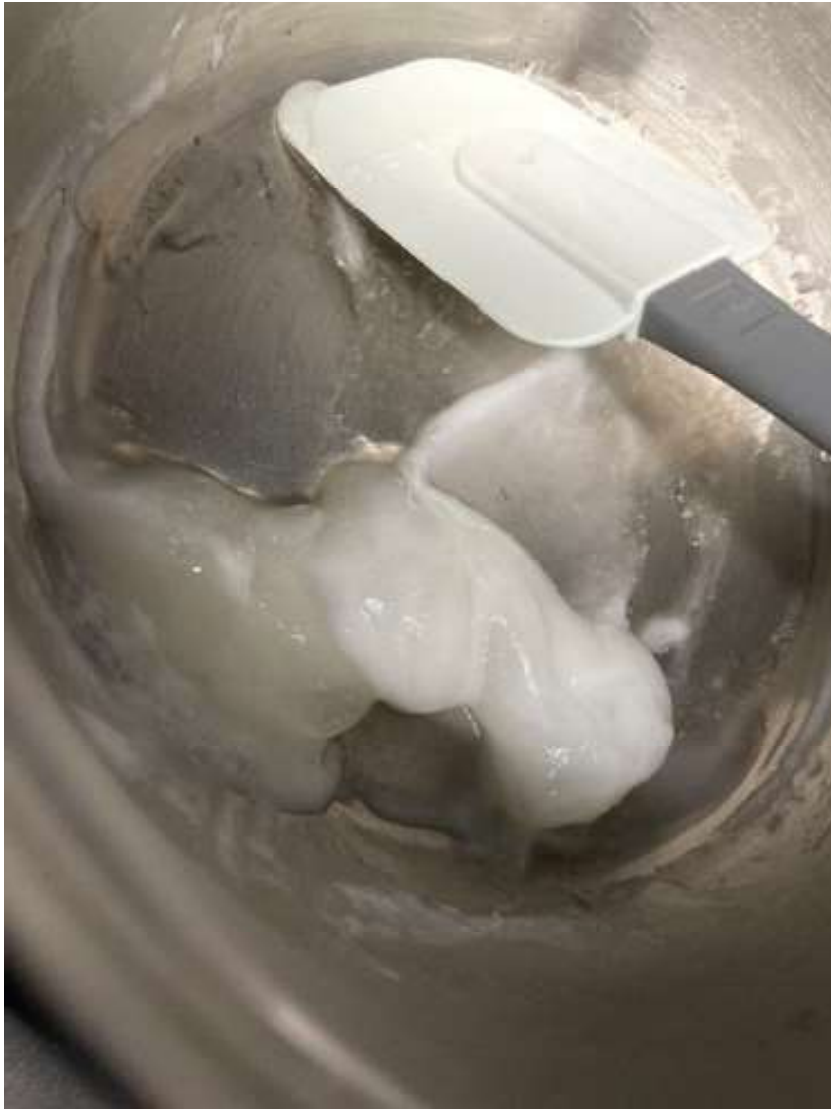
figure 41: Structure of the heated binder of 60 ml water and 5% beeswax
