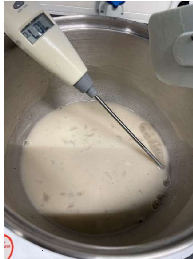
figure 12: Gel pockets at 70 degrees, but the rest is still liquid
