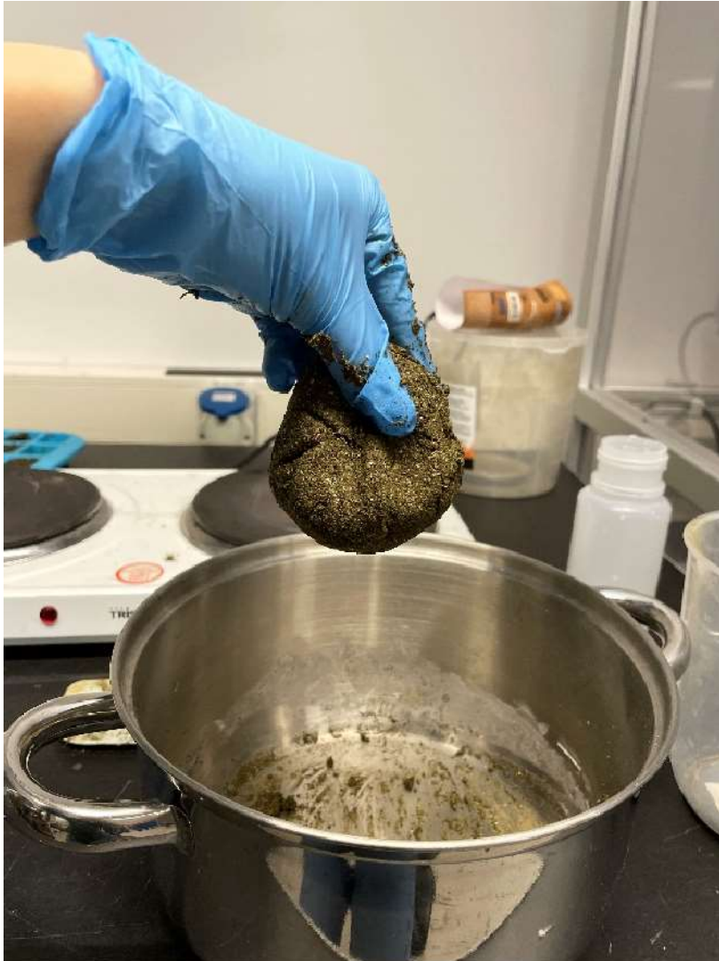
figure 43: The TeaClay had to be kneaded and moulded by hand. When the temperature was higher, the material was more sticky. After kneading several more times, it could form into one homogenous mass.
