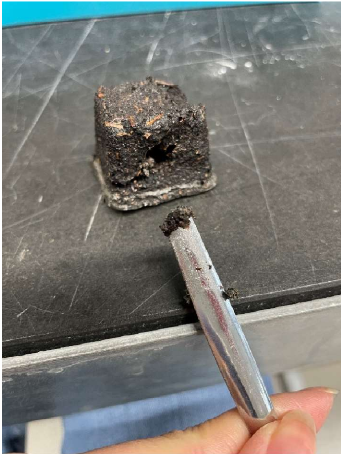
figure 37: Compared to gelatine that has not been in the oven, inside is not liquid, but it is like a paste.
