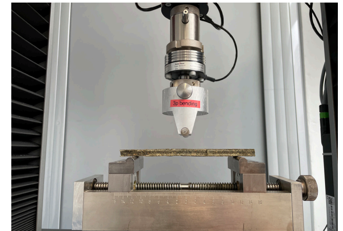
Figure 6.3: the test setup for the 3 point bending test.
