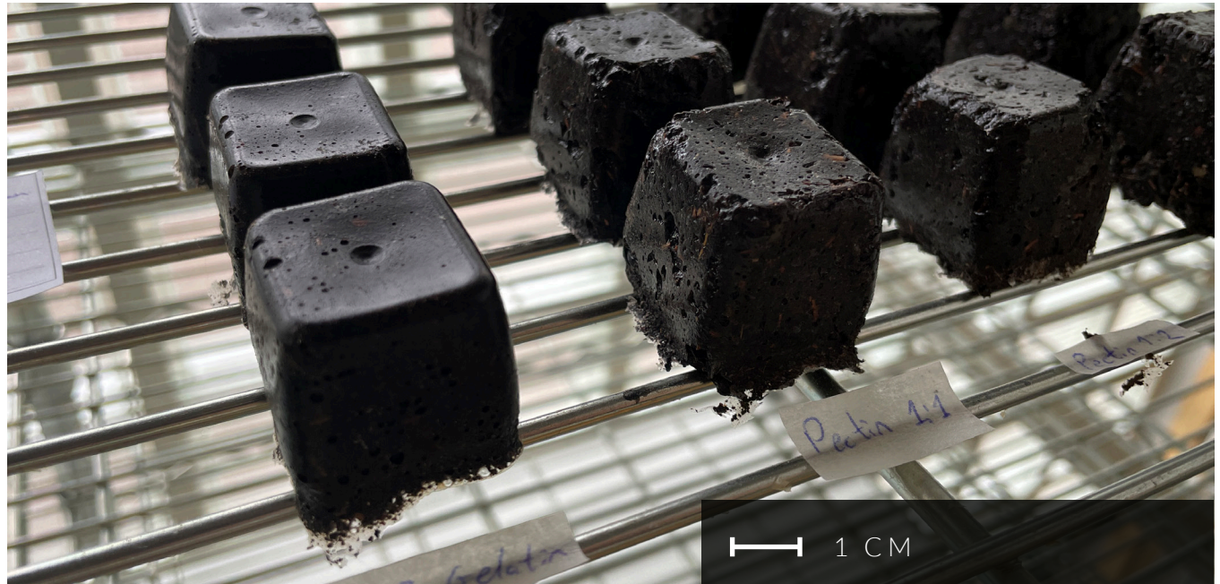
Figure 5.2: the fast demoulding of pectin and gelatine samples.
