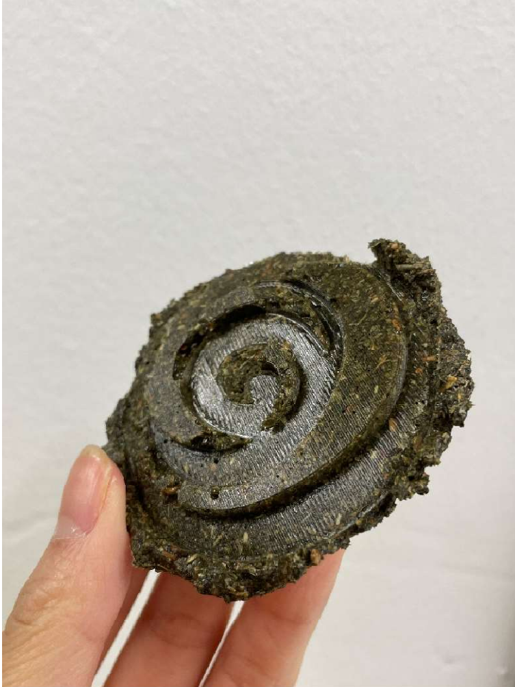
figure 69: the demoulded material conveyed the lines of the 3D printed mould.
