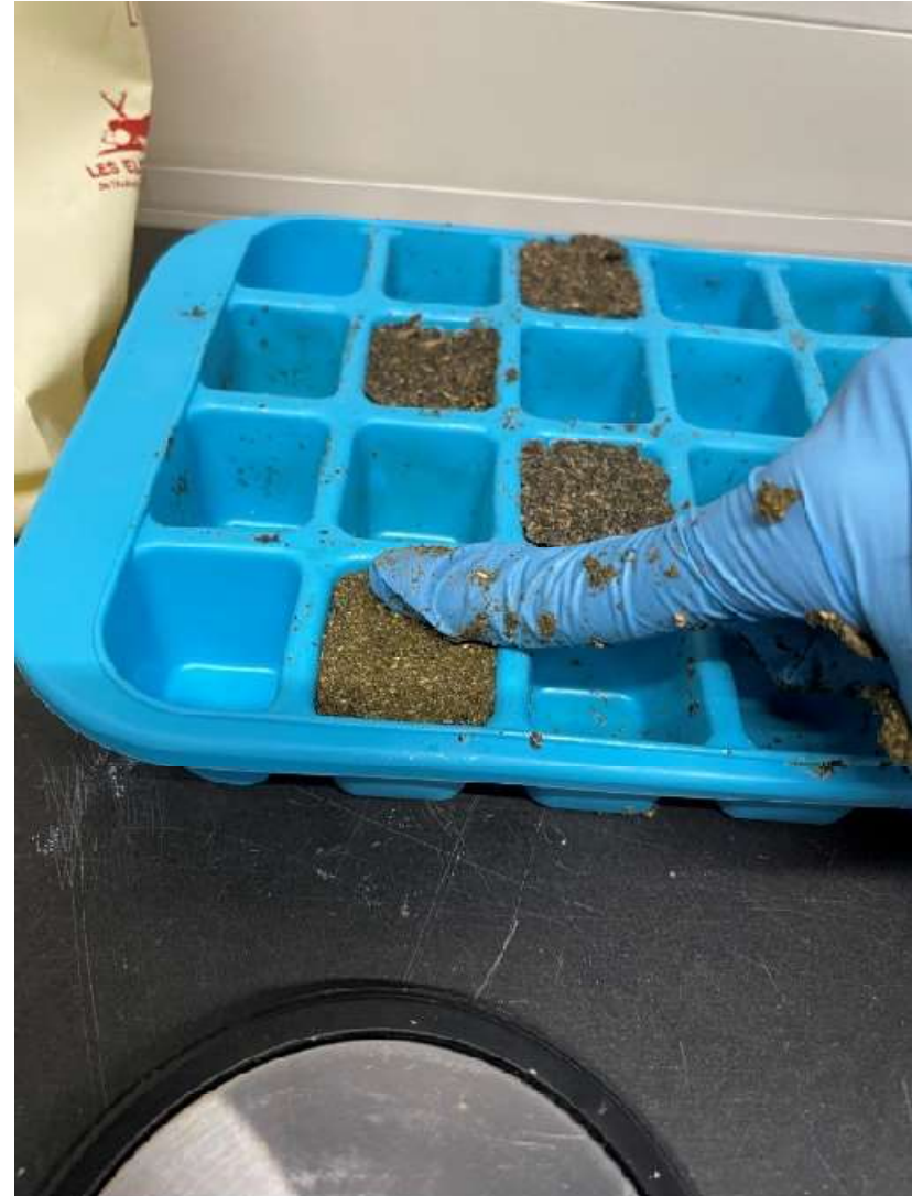
figure 44: The material had to be moulded by hand into the moulds
