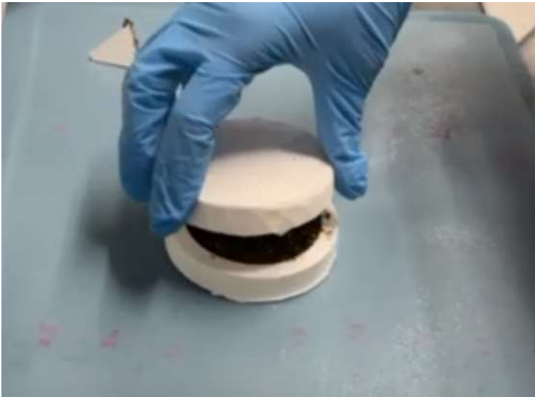
figure 63: pressing the tea clay with a mould.
