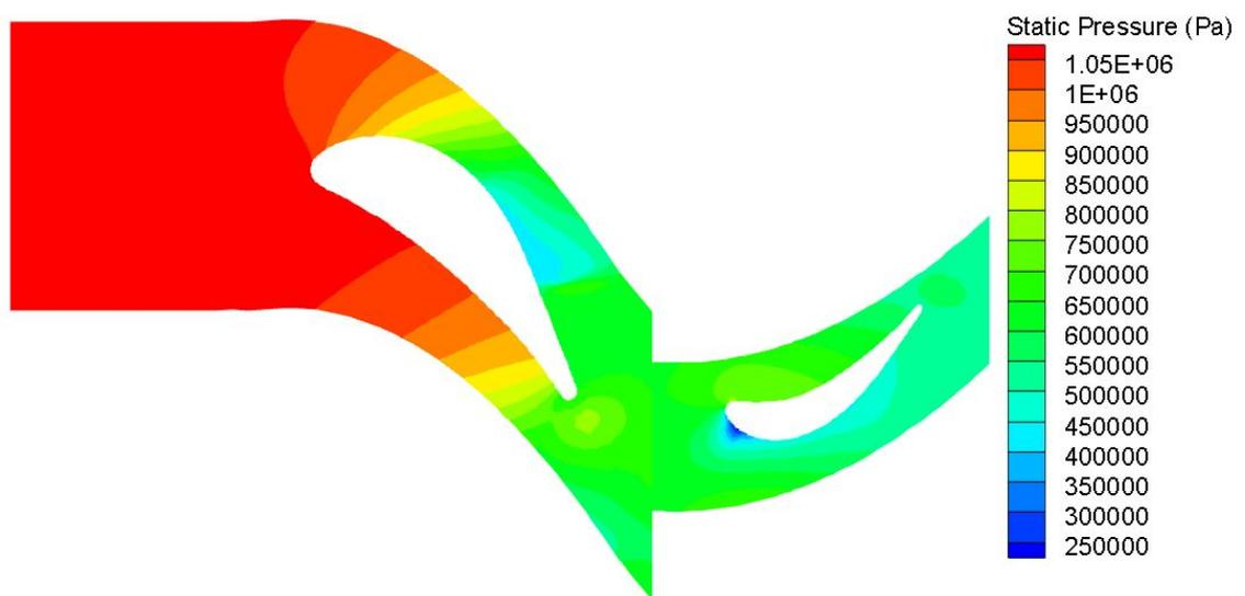
Figure 6.3: Static pressure distribution in the stage.
