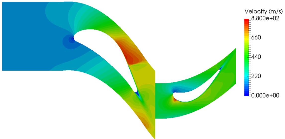
Figure 6.6: Velocity distribution in the stage
