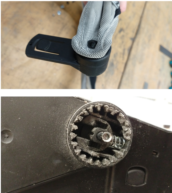
Figure 55. Two examples of parts from the second hand strollers’ disassembly. The top image shows the still good quality part of the seat’s cap. The bottom image shows dirt which got stuck in a mechanical part of the seat.
