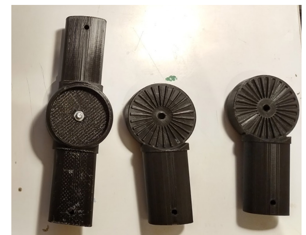
Figure 53. Development of key components for the reassembly from a stroller into a handcart and vice versa
