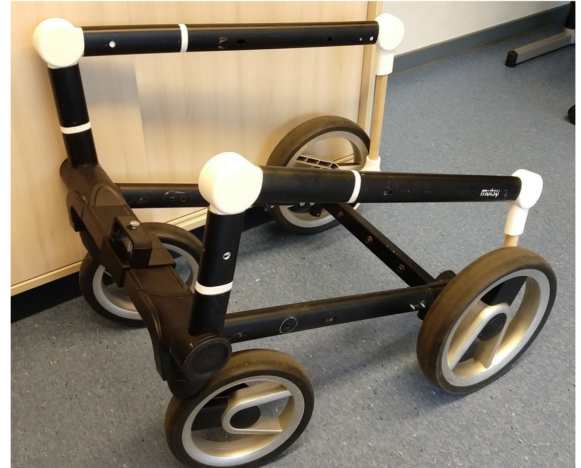
Figure 52. Proof of concept: a few key components can be used to reassemble the stroller components into a handcart and back.
