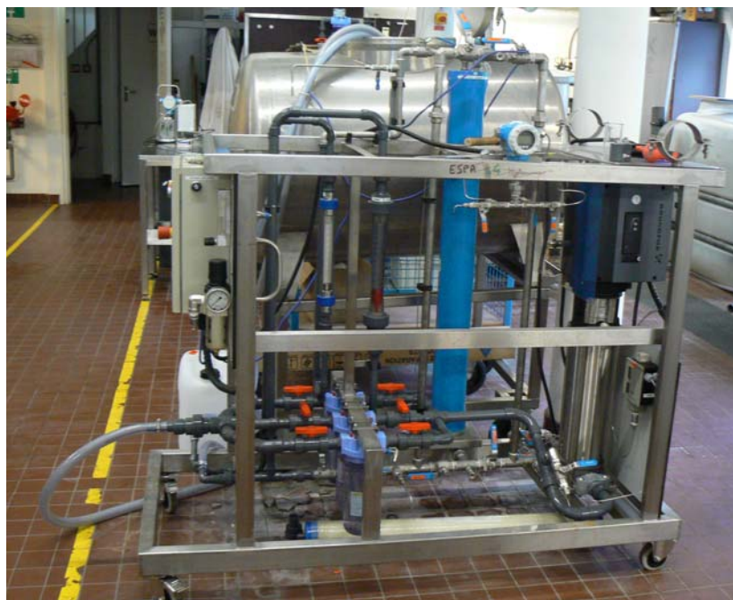
Figure 2.2 – Membrane filtration set-up for rejection experiments (in blue: membrane module)
