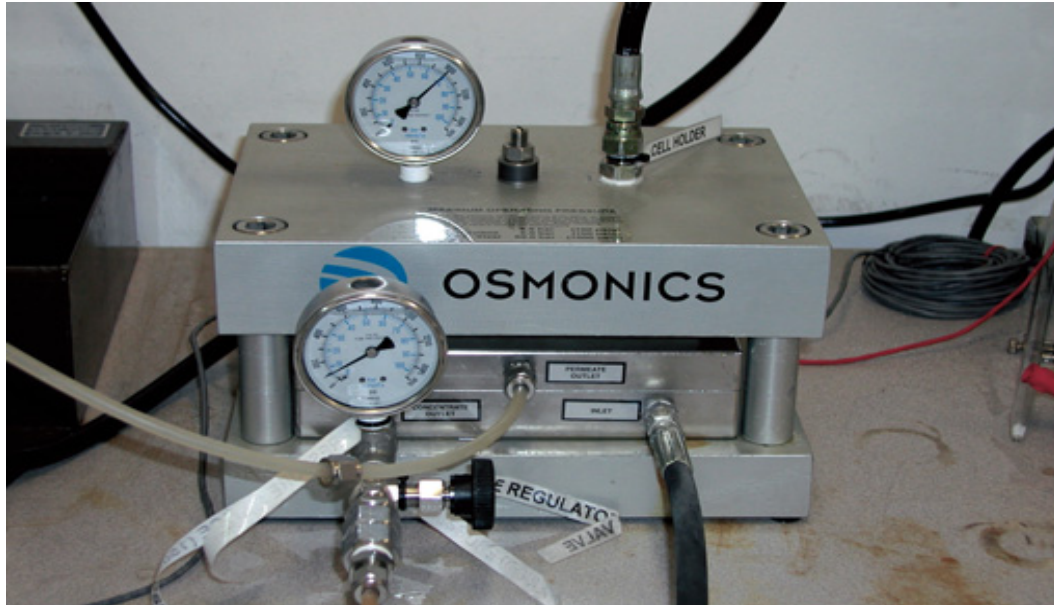
Figure 5.2 – Sepa CF II cross-flow membrane cell for fouling/rejection experiments
