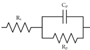
Figure 4.1. The equivalent circuit model representing the EIS response of the films (Park, et al., 2001)
