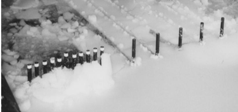
Figure 9. Difference in ice failure mode on  $l = 2D$  (left) and  $l = 8D$  (right) observed during physical model testing.
