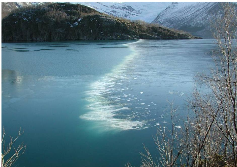
Figure 1. Surface disturbance from the bubble curtain in Holandsfjord (Eidnes, 2004). The brackish outflow is coming from the left.
