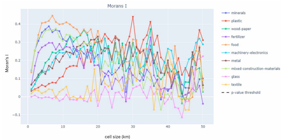
FIG. 5.7 Effect of cell size on Moran's I value. Line chart with cell size on the x-axis and Moran's I (strength of spatial clustering) on the y-axis. The chart shows, for each material, how strongly waste reuse locations are clustered at each cell size
