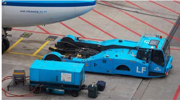
Figure 5-12. GPU and push/pull tractor (NACO Aviation Academy, 2023d).
