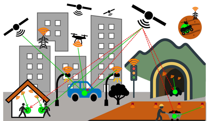
FIGURE 1. Overview of PL positioning in GNSS-obstructed and denied environments, including urban areas, indoors, tunnels, underground, and on Mars. Orange icons are PL transmitters, and green dots are receivers.
