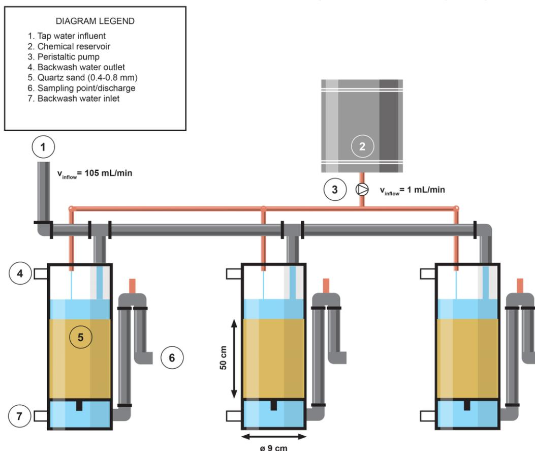
Figure 2: Schematic overview of filter columns
