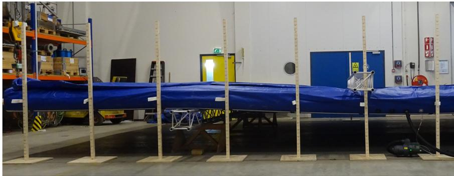
Figure A.1: A photograph of the test setup showing the gauge rods (courtesy of TNO).
