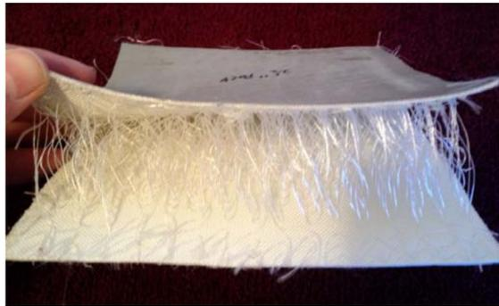
Figure 1.3: An example of a polyester drop-stitch fabric with coated rubber skins [24]
