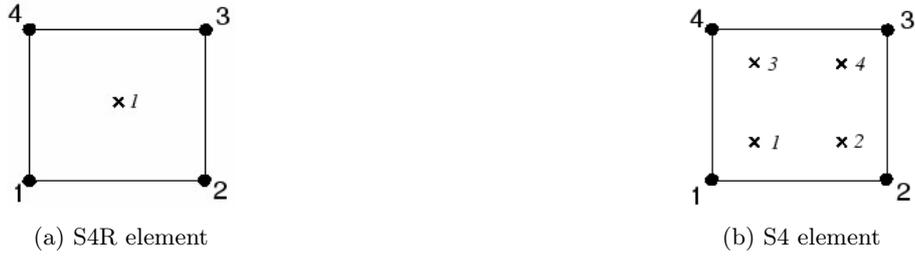
Figure 3.1: A depiction of the integration points of fully integrated linear shell element (S4) and reduced integrated shell element (S4R) [76].
