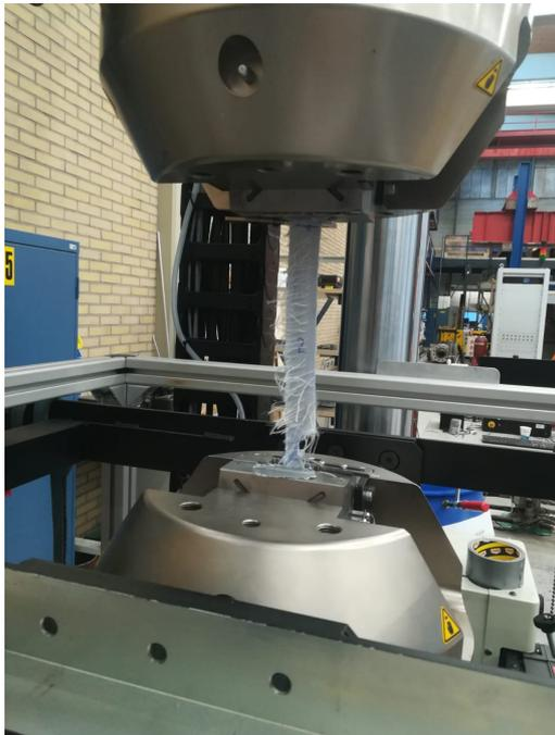
Figure 5.6: An example of a specimen broken near the grips
