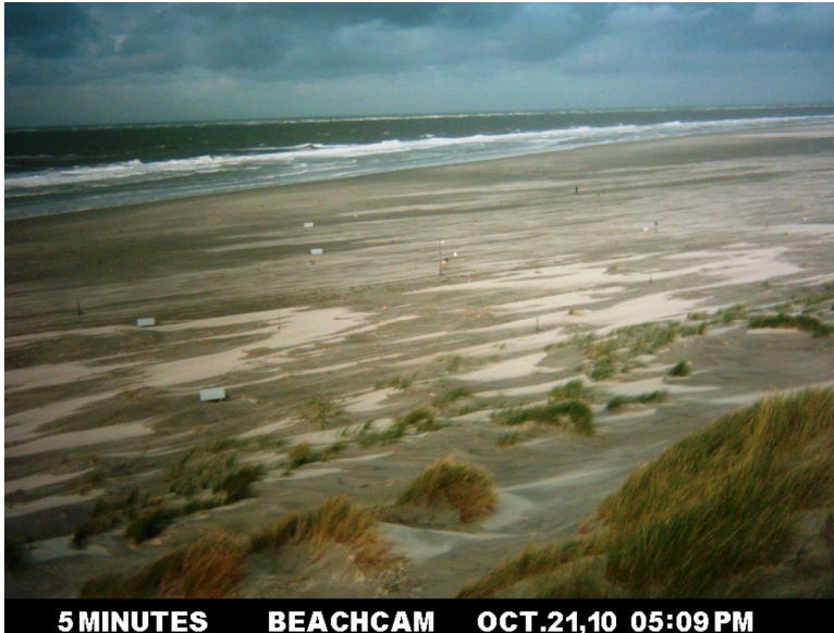
Figure 3.7 Field-work location at Ameland, The Netherlands. The dry and moving sand (light) contrasts with the more moist beach surface (dark). The grey boards were used as a spatial and colour reference. The 'Beach cam' took a picture every 5 minutes to monitor the continuously changing beach surface and visualise dune development.
