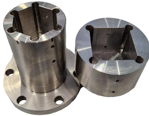
Figure 10. Image of the steel holders. On the left the top part of the steel holders with the hexagonal prism and on the right the bottom part with the square prism.
