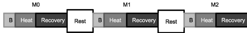
Fig. 1. Protocol timeline. After a 15 min acclimation period, the measurements start. One measurement consists of three phases: the baseline (B, 1 min), heating phase (up to 42 °C) and a recovery phase (9 min), followed by a 5 min rest. The measurements are executed in cycles of 3 measurements.
