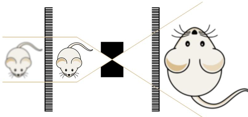
**Figure 2.2:** Schematic of the projection of a mouse by means of a parallel-hole collimator only (left-hand side) and by means of a combination of a parallel-hole collimator and a pinhole collimator (right-hand side).
