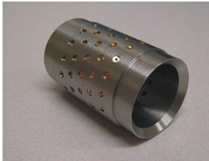
**Figure 2.3:** A cylindrical multi-pinhole collimator with 75 pinholes. Image taken from Van der Have [27].
