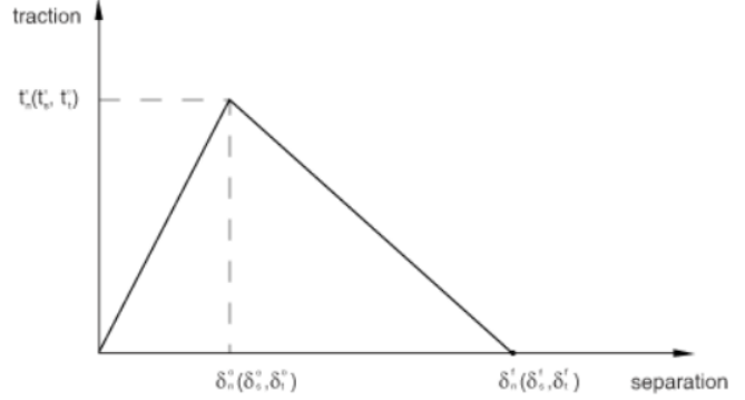
Figure 2.9: Abaqus bi-linear cohesive damage law [34]
