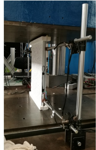
Figure 5.10: LVDTs mounting support and location
