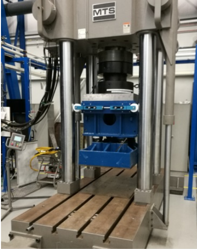
Figure 5.19: MTS3500 compression testing machine at the TUD ASM lab
