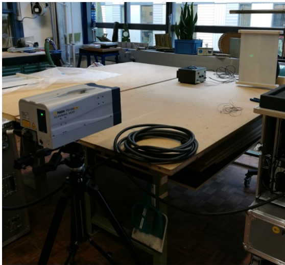
Figure C.1: Test set-up used to measure the panel with tabs frequency response
