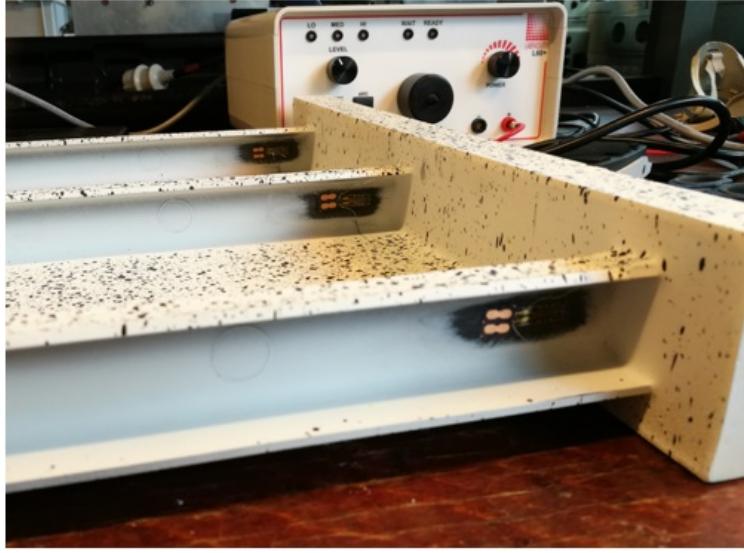
Figure 5.8: Web strain gauges mounted on the panel
