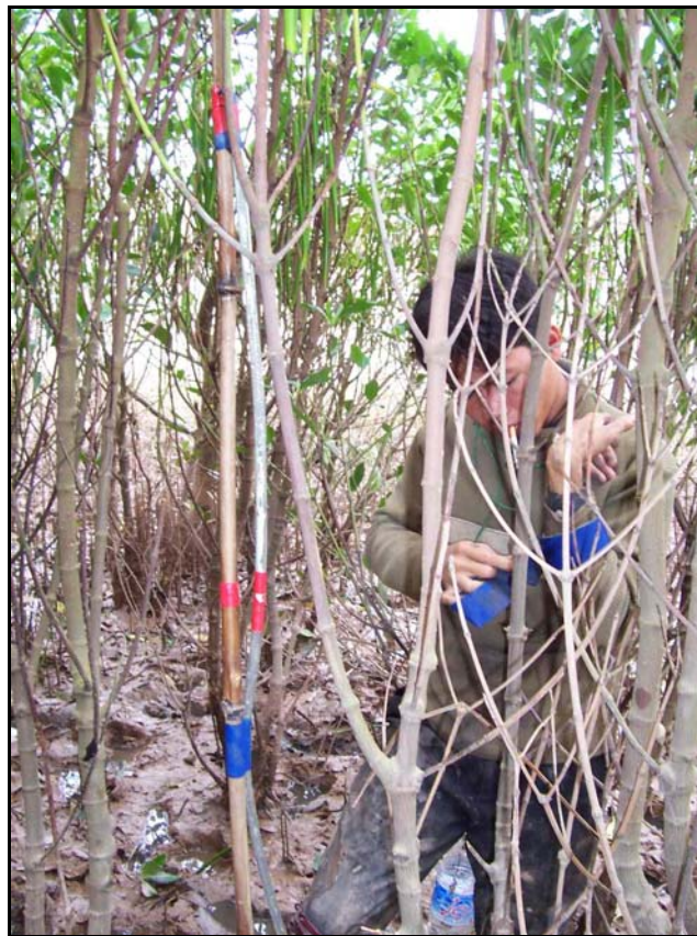
Figure 9.4 Highly mobile level instrument in dense forest
