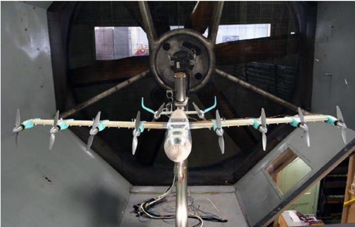
Figure 17: GL-10 28.125% scale tunnel model in NASA Langley's 12-foot Low Speed Wind Tunnel, 9-inch diameter Propeller and a wingspan of 10.5 ft [Ref.41]
