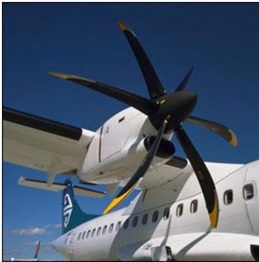
Figure 19: Hamilton standard 568F propeller mounted on Pratt & Whitney Pw100 engine on an ATR72 [Ref.45]
