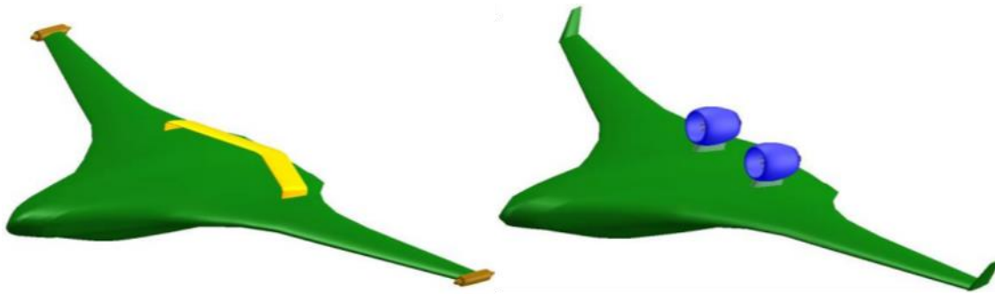
Figure 4: on left: N3-X FLOPS Model with distributed propulsion system on right: N3A FLOPS Model with pylon and nacelle configuration [Ref.12] FLOPS: Flight Optimization System Developed by NASA
