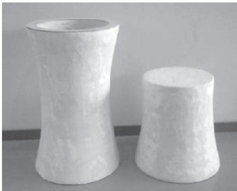
Figure 7-18 Foam prototype of the first splash design.
