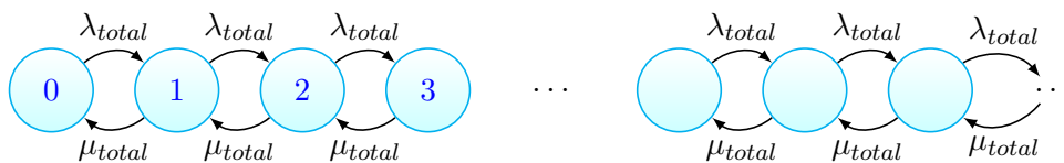
Figure 3-8: Markov Chain describing the network part of the multiple user scenario with one cloud.
