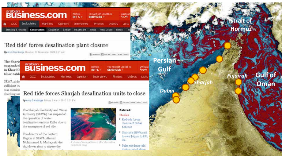
Figure 1-7: The massive red tide bloom in the Gulf of Oman as shown in this satellite image acquired by Envisat's MERIS instrument on November 22, 2008 (Credits: C-wams project, Planetek Hellas/ESA). Yellow points indicate location of large SWRO plants in the area. Inset screenshots of online news regarding SWRO plant shutdown due to red-tide in the gulf in 2008 and 2013 ( www.arabianbusiness.com ).
