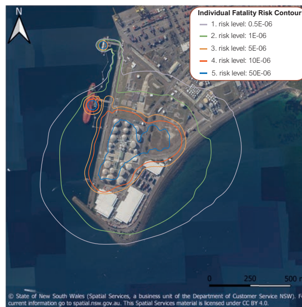
Figure 2.3: Individual fatality risk contours for an oil terminal, Port Botany, Australia (source: Spatial Service State of New South Wales, contours from Sherpa consulting , image by TU Delft – Ports and Waterways is licenced under CC BY-NC-SA 4.0).
