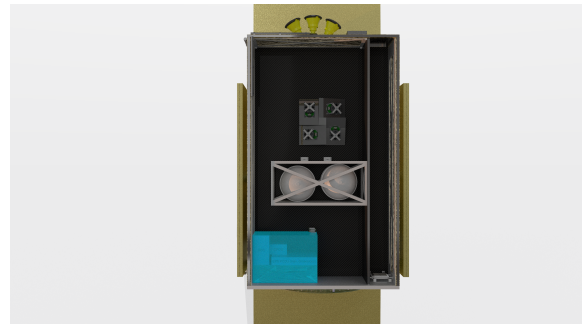
Figure 15.2: Front view of the NEBULA-Xplorer's internal architecture
