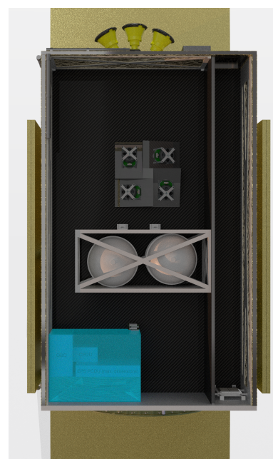
Figure 14.1: Reaction Wheel Module and Propulsion system structures in the spacecraft
