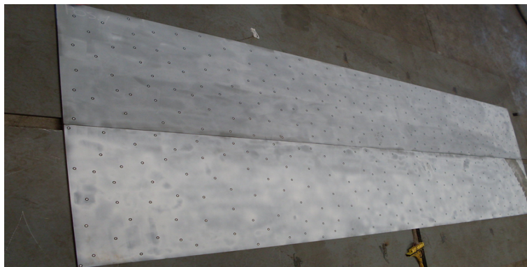
Figure 7.3. Two plates of AH36 with dimensions of 3600 \times 600 \times 6 \text{ mm}^3 used in the SAW process. The plates are painted, in order to measure the out-of-plane deformation.
