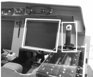
Figure B.2: An illustration of experimental devices. The side-stick and the LCD screen are marked by rectangles. The side-stick could be moved around the roll axis (left/right). The headphone used in the experiment is not shown in this figure.
