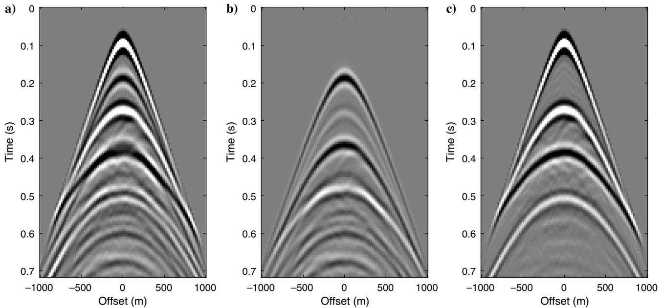
Figure 2. Modeled reference data. (a) True full waveform. (b) True multiples. (c) True primaries.
