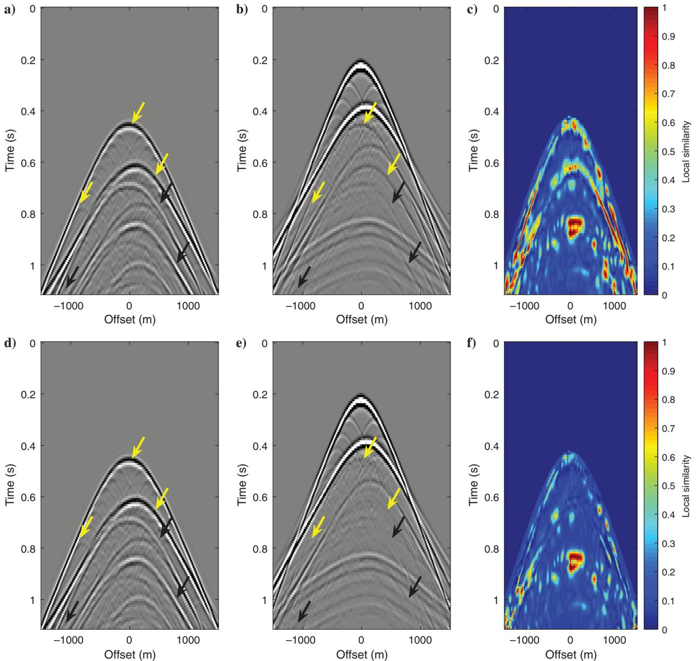
Figure 10. (a and b) Initially predicted multiples and primaries using conservative SRME with a global subtraction window, respectively. (d and e) Final estimated multiples and primaries after LPMO, respectively. (c and f) Local similarity maps before and after LPMO, respectively. The yellow arrows indicate where the leaked multiples are extracted, and the black arrows indicate where the phase-shift leaked multiples are extracted.
