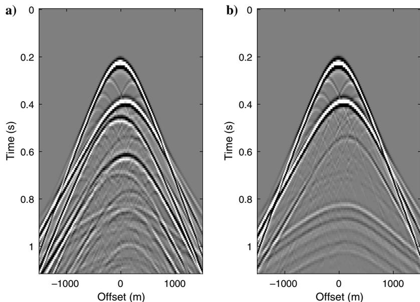
Figure 8. Modeled reference data. (a) True full wavefield after deghosting. (b) Reference primaries.
