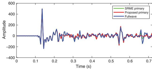
Figure 16. Single-trace comparison at offset 87.5 m before and after LPMO. The blue line denotes the full wavefield, the green line denotes the conservative SRME primaries, and the red line denotes the proposed primaries after LPMO.
