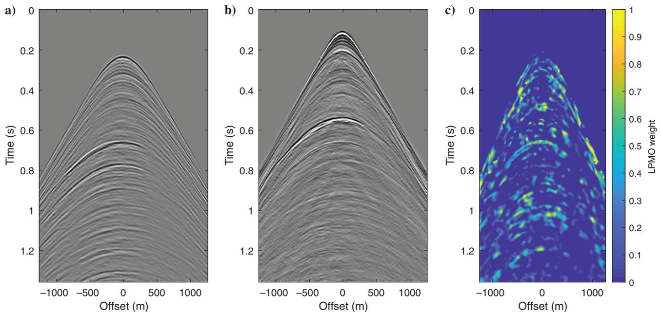
Figure 14. Initially estimated (a) multiples and (b) primaries using conservative SRME with large subtraction windows. (c) The estimated LPMO weight based on (a and b). The surface-related multiple leakage can be effectively detected by the LPMO weight.
