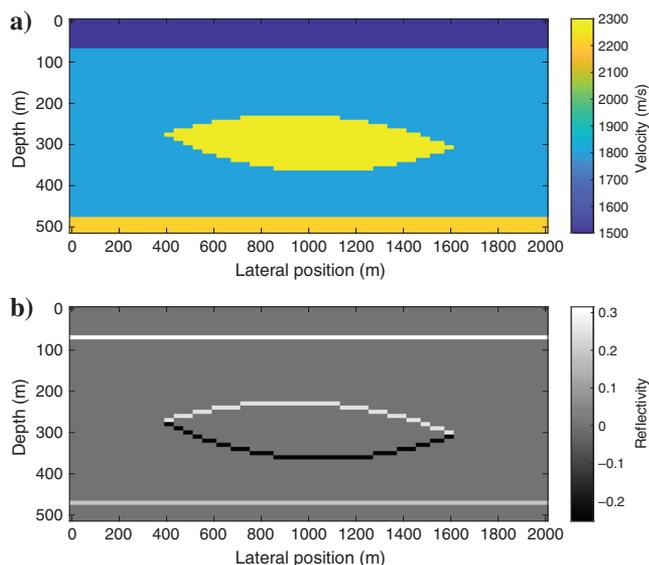
Figure 1. A 2D lens-shaped synthetic model. (a) Velocity model. (b) Reflectivity model.
