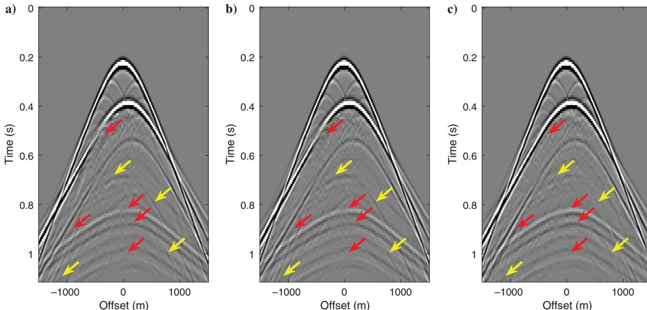
Figure 12. Comparison to the standard SRME. (a)  $L_2$ -norm standard SRME primaries with a 320 ms \* 25 traces local subtraction window size. (b)  $L_1$ -norm standard SRME primaries with a 320 ms \* 25 traces local subtraction window size. (c) The proposed primaries after LPMO (for comparison purposes). The yellow arrows in (a and b) denote the more severe multiple leakage compared to those in (c). The red arrows in (a and b) denote the primary damage compared to those in (c).
