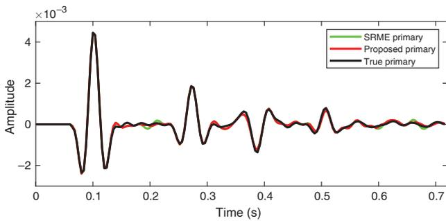
Figure 5. Single-trace comparison before and after LPMO. The black line denotes the true modeled primaries, the green line denotes the conservative SRME primaries, and the red line denotes the proposed primaries after LPMO.
