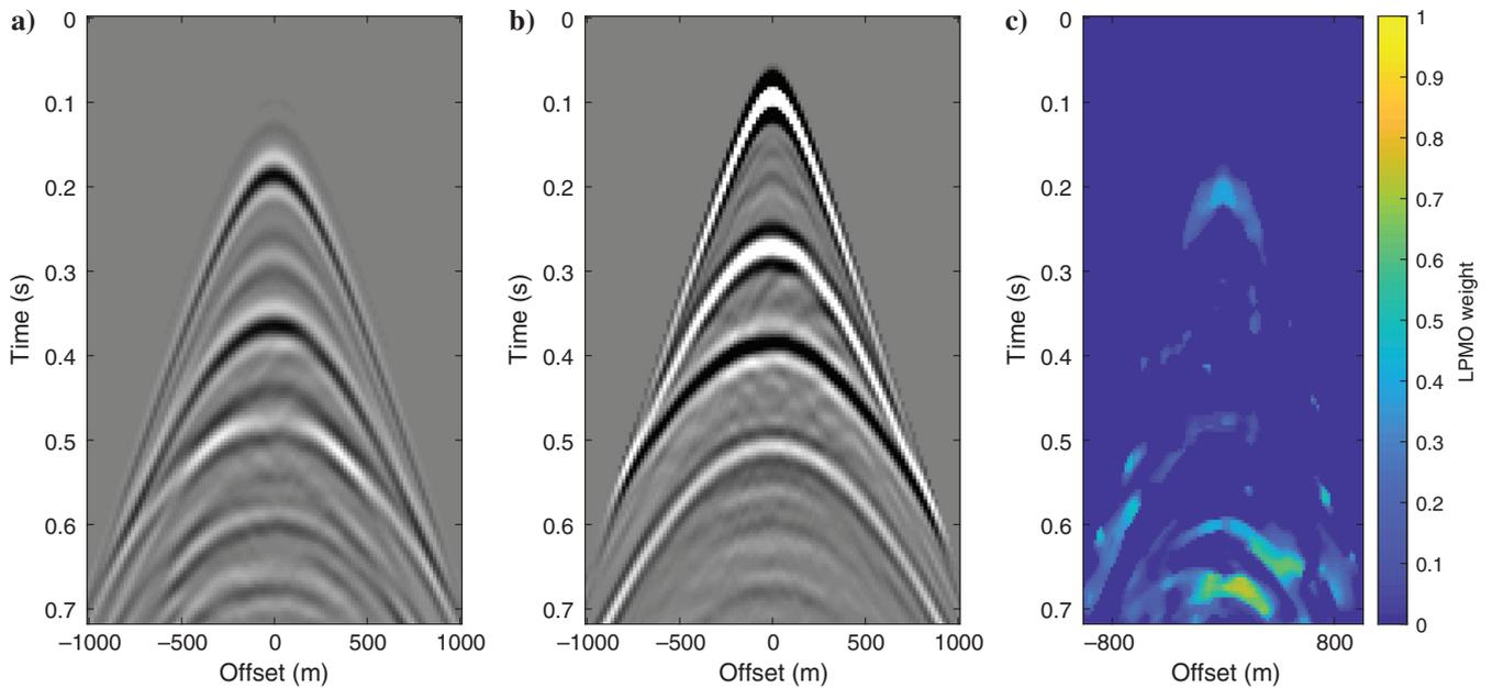
Figure 3. Initially predicted (a) multiples and (b) primaries using conservative SRME with a global subtraction window. (c) The estimated LPMO weight based on (a) and (b). The surface-related multiple leakage can be effectively detected by the LPMO weight.
