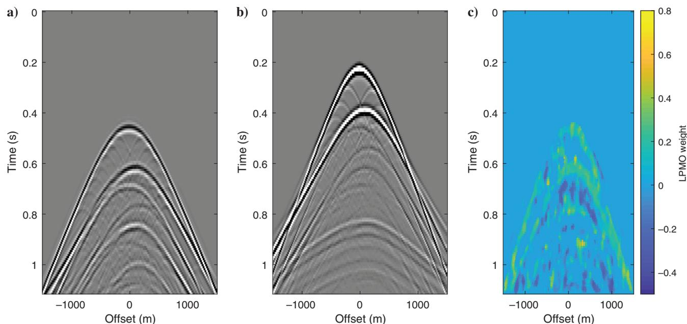
Figure 9. Initially predicted (a) multiples and (b) primaries using conservative SRME with a global subtraction window. (c) The estimated LPMO weight based on (a) and (b). The surface-related multiple leakage can be effectively detected by the LPMO weight. Note that the negative weights come from phase-shift errors during conservative SRME.
