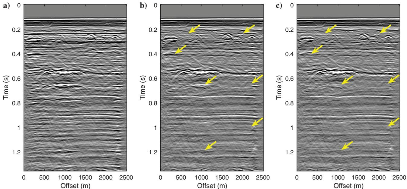
Figure 18. Stacked section comparison. (a) Stacked section of the input. (b) Stacked section of the initially predicted primaries by conservative SRME with large subtraction windows. (c) Stacked section of the final estimated primaries after LPMO.
