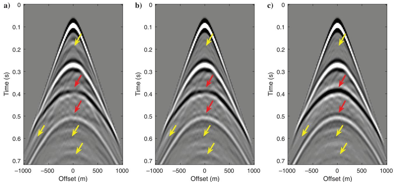
Figure 6. Comparison to the standard SRME. (a)  $L_2$ -norm standard SRME primaries with a 240 ms \* 25 traces local subtraction window size. (b)  $L_1$ -norm standard SRME primaries with a 240 ms \* 25 traces local subtraction window size. (c) The proposed primaries after LPMO (for comparison purposes). The yellow arrows in (a and b) denote the more severe multiple leakage compared to those in (c). The red arrows in (a and b) denote the primary damage compared to those in (c).
