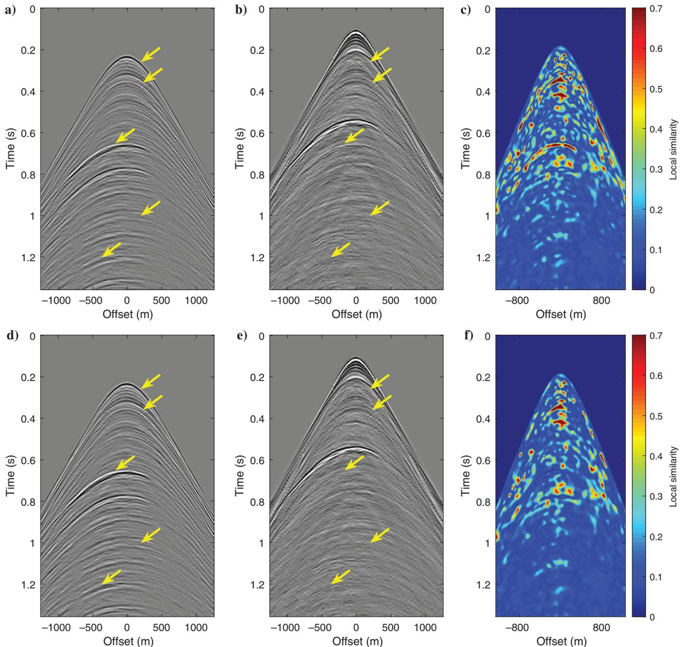
Figure 15. (a and b) Initially predicted multiples and primaries using conservative SRME with large subtraction windows, respectively. (d and e) Final estimated multiples and primaries after LPMO, respectively. (c and f) Local similarity maps before and after LPMO, respectively. The yellow arrows indicate where the leaked multiples are extracted.
