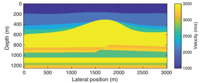
Figure 7. Complex salt velocity model.
