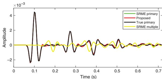
Figure 21. Single-trace comparison before and after LPMO from the lens-shaped synthetic model.
