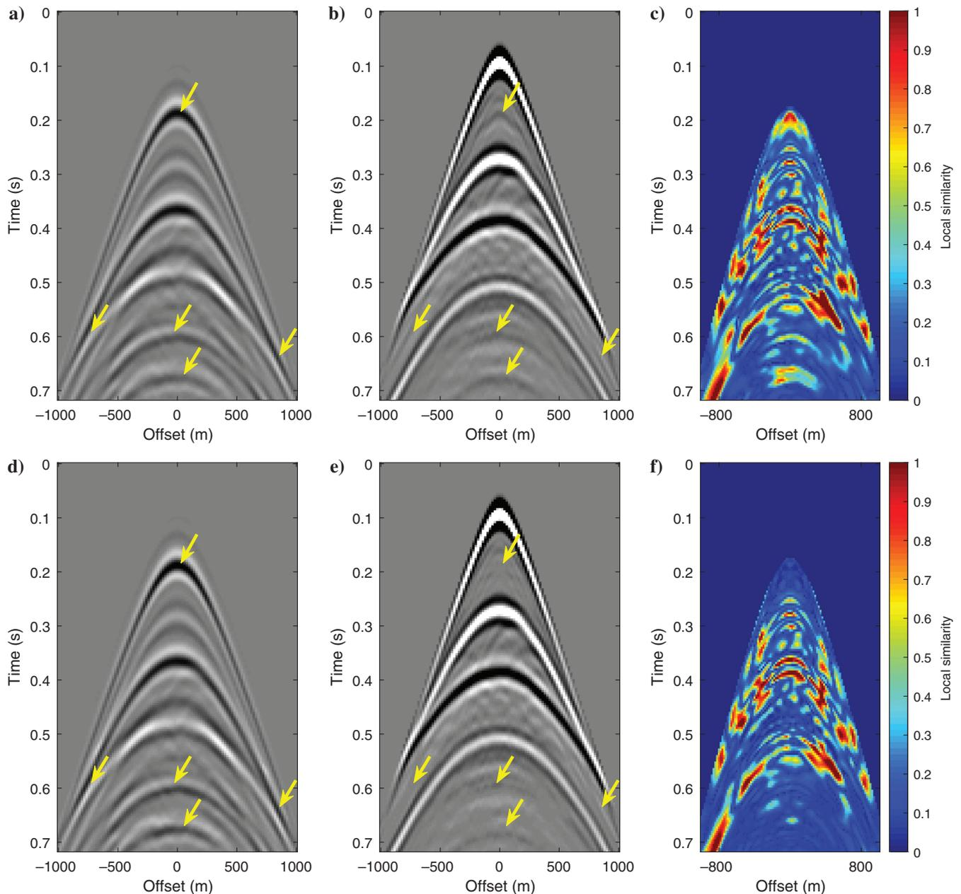
Figure 4. (a and b) Initially predicted multiples and primaries using conservative SRME with a global subtraction window, respectively. (d and e) Final estimated multiples and primaries after LPMO, respectively. (c and f) Local similarity maps before and after LPMO, respectively. The yellow arrows indicate where the leaked multiples are extracted.
