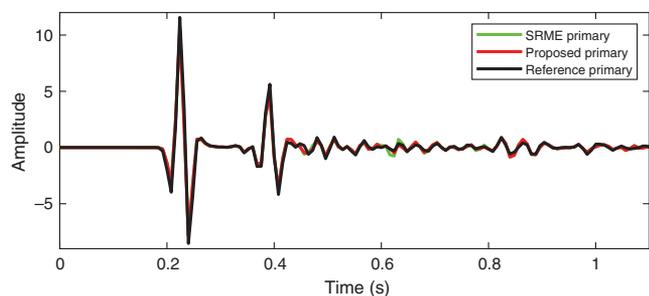
Figure 11. Single-trace comparison before and after LPMO. The black line denotes the reference primaries, the green line denotes the conservative SRME primaries, and the red line denotes the proposed primaries after LPMO.
