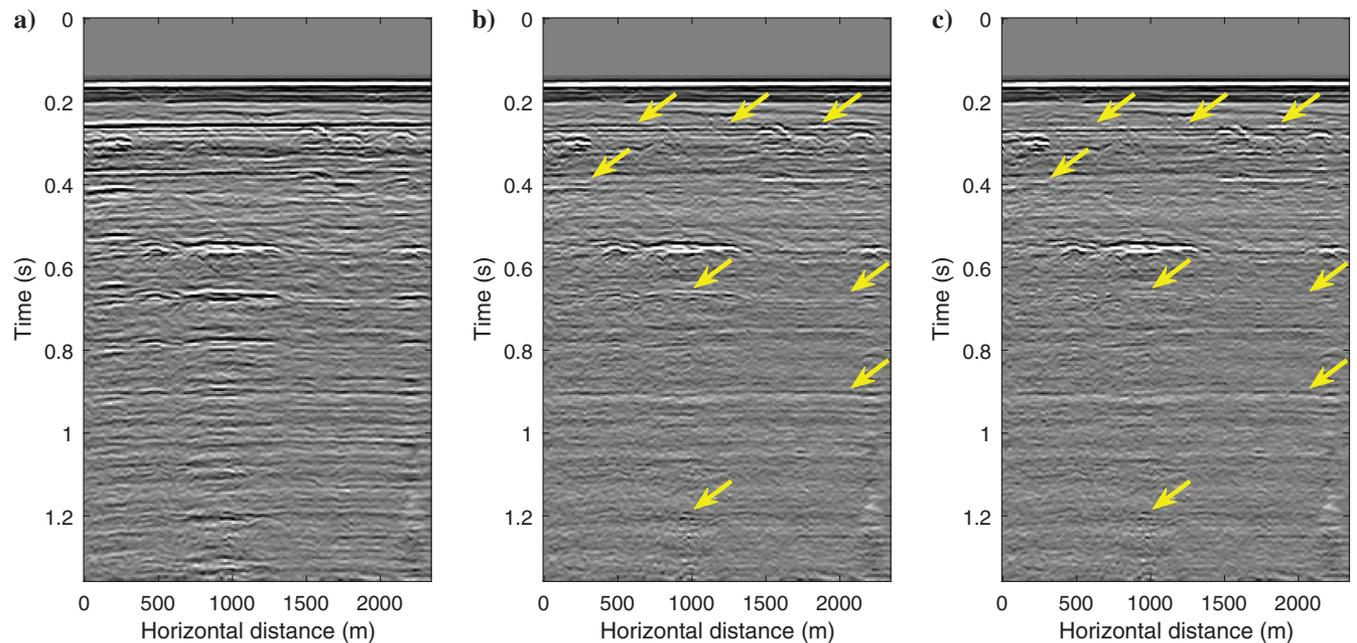
Figure 17. Common-offset gather comparison at offset  $-150$  m. (a) Common-offset gather of the input. (b) Common-offset gather of the initially predicted primaries by conservative SRME with large subtraction windows. (c) Common-offset gather of the final estimated primaries after LPMO.
