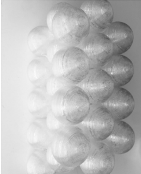
FIG. 7 3d-printed model Left: Insulation spheres Right: with triangular plates
