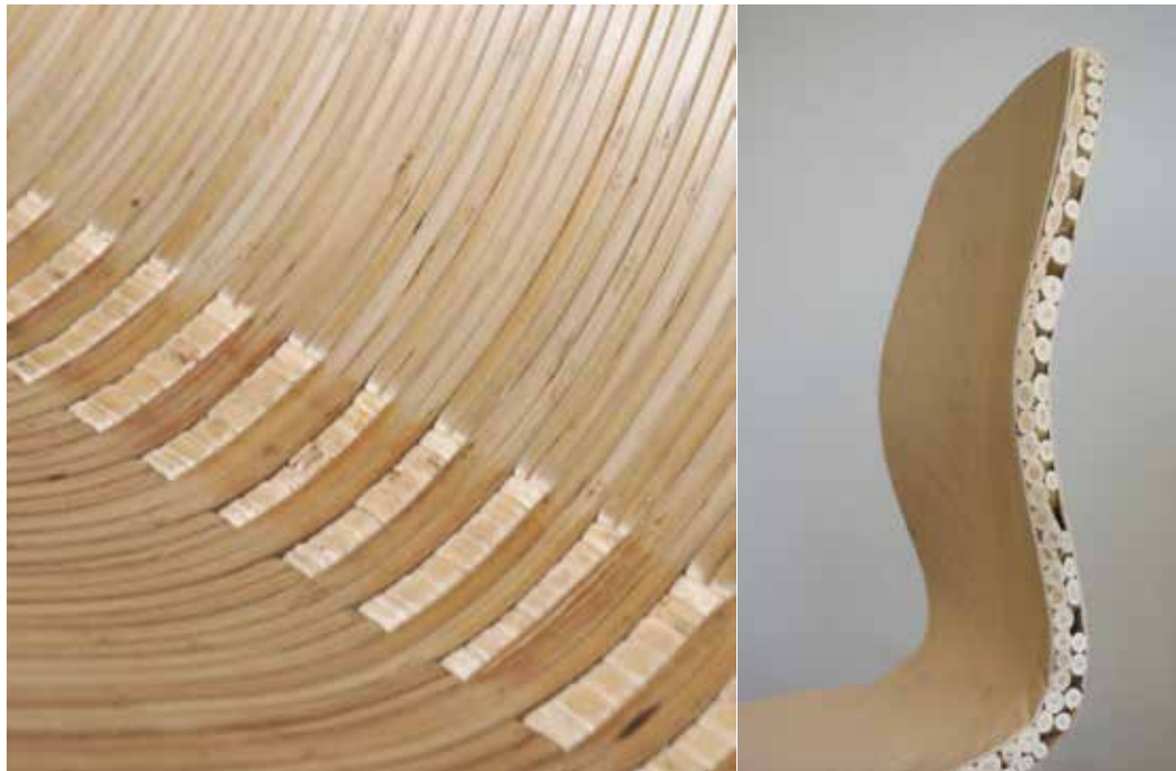
FIG. 10 SALIX REGIONALIS 3D is a new lightweight construction material made from willow, R&D: BAU KUNST ERFINDEN // BUILDING ART INVENTION, University of Kassel, S. Silbermann, T. Klooster, J. Juraschek, D. Becker and H. Klussmann, funded by the BMWi/ ZIM, Photo:BAU KUNST ERFINDEN
