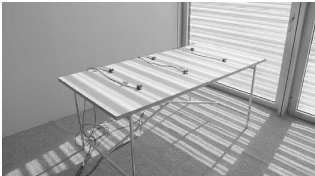
FIG. 7 measurements to the visual comfort: levels of illuminance
