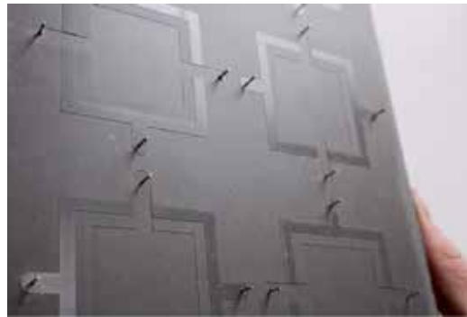
FIG. 4 Prototype of the electric system of a DysCrete- Solar Concrete - PV-Panel R&D: BAU KUNST ERFINDEN // BUILDING ART INVENTION, University of Kassel, T. Klooster, S. Aden, J. Iwanowicz and H. Klusmann, funded by the Forschungsinitiative Zukunft Bau/ BBSR, Photo: BAU KUNST ERFINDEN
