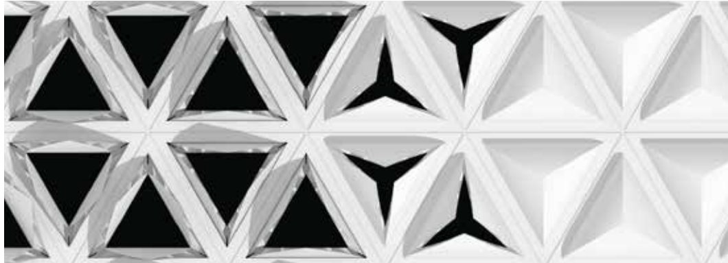
FIG. 13 Pyramid modules of hingeless façade openings
