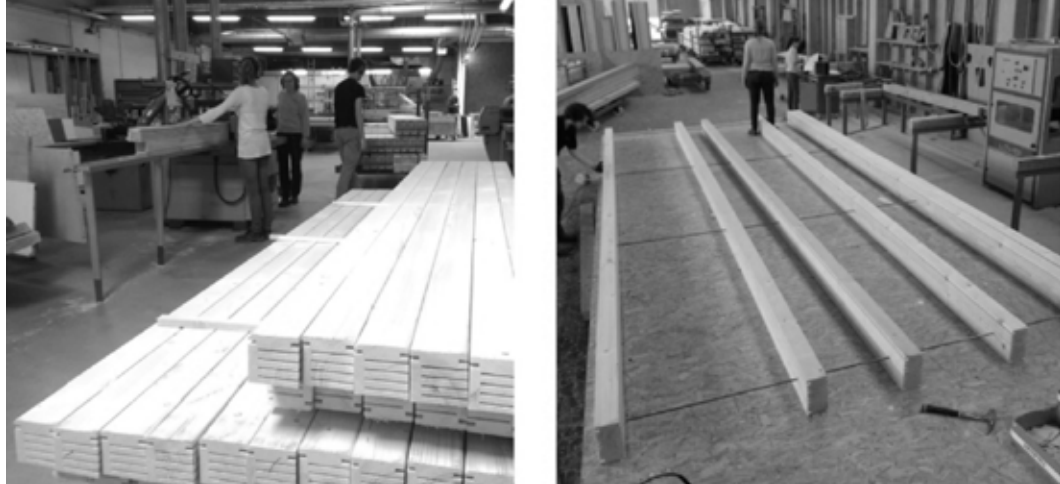
FIG. 4 Elements being assembled into a wall segment (photographed by Hans Drexler and Alexander Quiring, MSA 2012)
