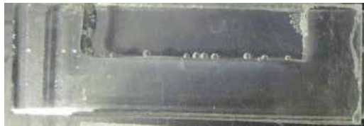
FIG. 4 Transparent Structural Sealant after 10000 hours UVA exposure
