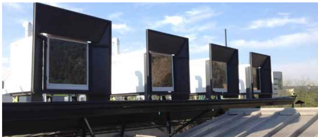
FIG. 7 Diagram showing the parts of the test chambers (top left) and layout of four chamber, three for testing sun protections plus one control chamber on the test platform (top right) and image of the built chambers (bottom)
