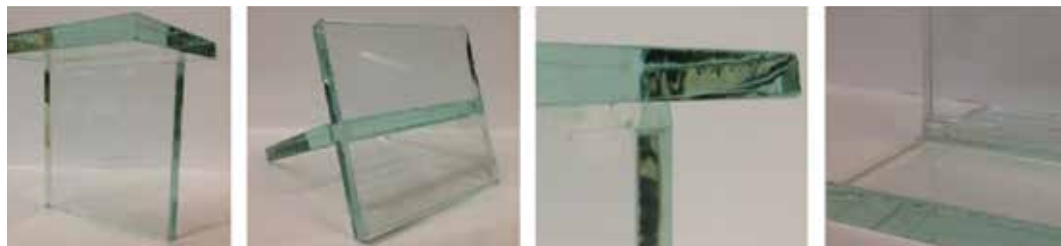
FIG. 8 Aesthetics in glassfin fixation using transparent structural silicone adhesive
