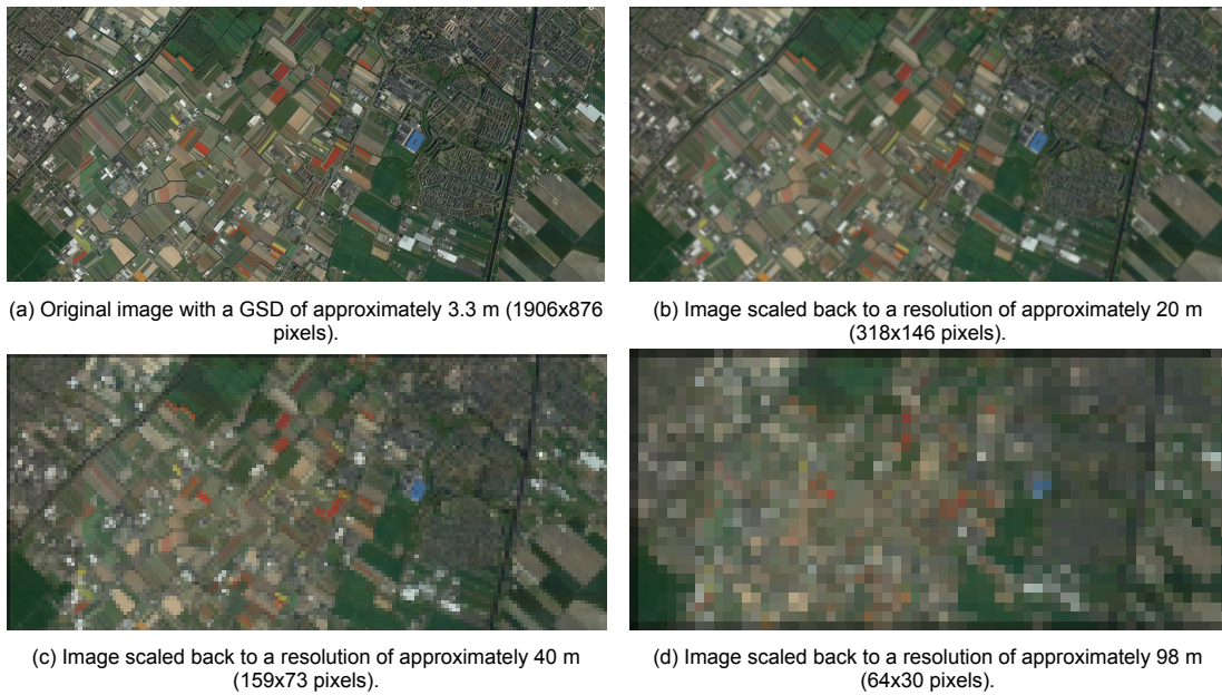
Figure 3.6: Aerial images of the fields south of Lisse scaled back to different resolutions. The border artifacts are caused by the convolution used to calculate down-sampled pixel values (image source: Google Earth).
