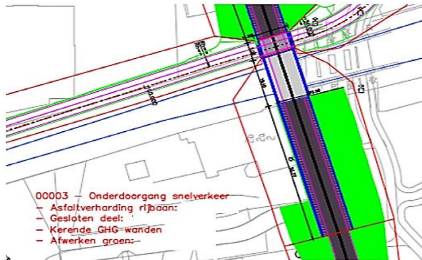
Figure 6.3 Example of the design of cost driving component with boundaries and tagged information
