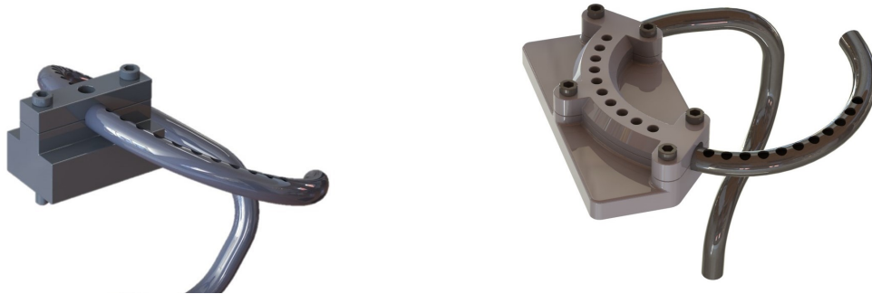
Figure D.7: The drill jigs for creating the camera hole (left) and the twenty holes for lighting (right).
