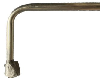
Figure D.6: Flattening of the tube after bending with a 30 mm radius.
