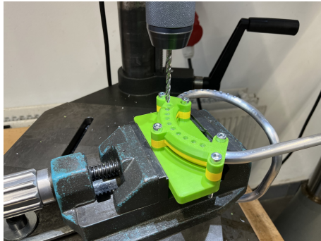
Figure 11.7: The drill jig for the twenty lighting holes.
