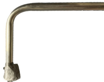
Figure 11.6: Flattening of the tube after bending with a 30 mm radius.
