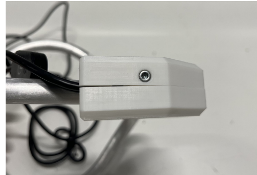
Figure 11.8: The gap in between the two housing parts.
