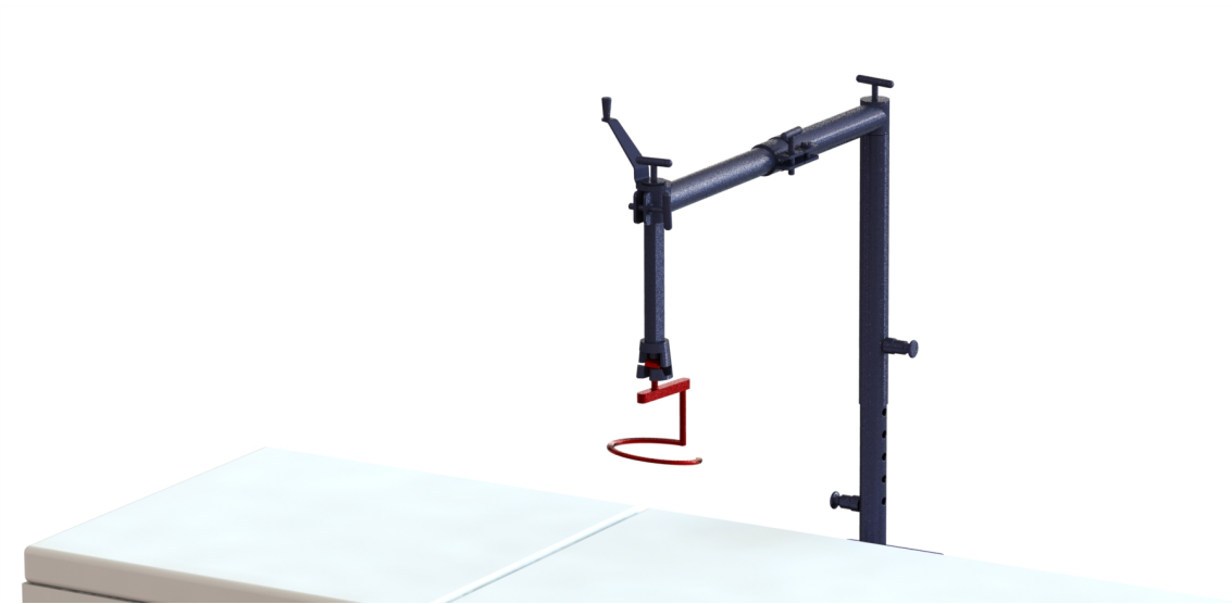
Figure 2.2: A render of the RAIS AWL system. The red part is the lifting device, which is connected to the retractor arm.
