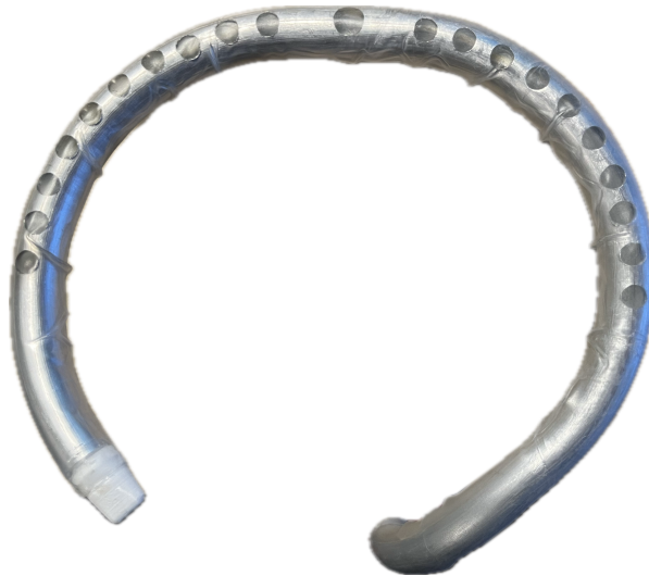
Figure 11.10: The wrinkles and scratches on the heat shrink.
