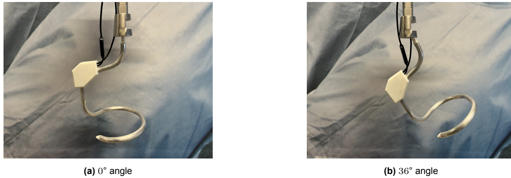
Figure 14.2: The incremental pitch, altering the camera angle.
