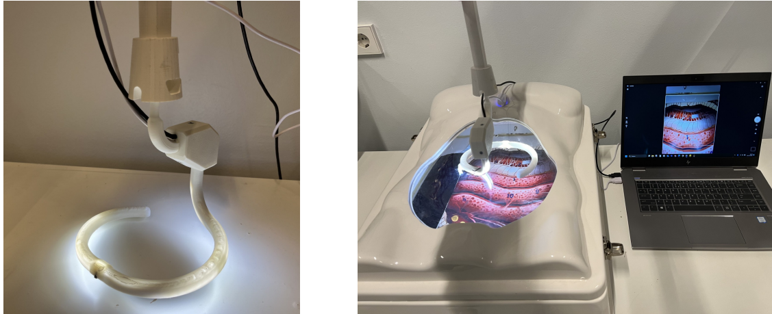
Figure 11.2: The 3D-printed prototype connected to the RAIS retractor arm.
