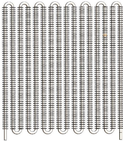
Figure 6.2.28 – single tube lay-out of one heating element.
