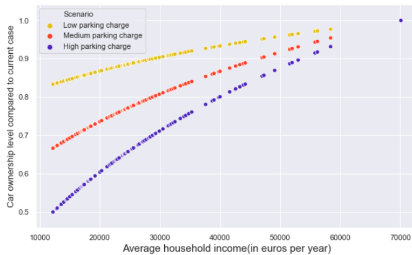
Figure 5.10: Car ownership reduction and its relation with income per household under different policy scenarios
