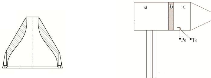
Figure 9.1 Left: contoured nozzle; right: schematic of the nozzle mount
