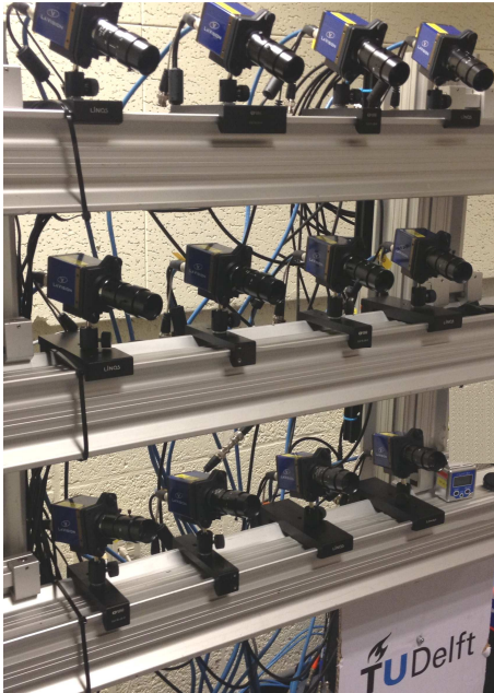
Figure 9.5 4-pulses TOMO PIV; left) imaging system used in the experiment on high speed separated flows (courtesy of K. Lynch); (right) sketch of the acquisition process using tomographic systems T1, T2 and T3 and lasers L1 and L2
