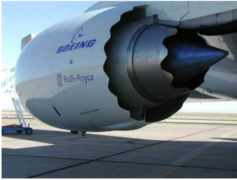
Figure 2.11 Chevron geometry of Rolls Royce engine on Boeing 777-200ER
