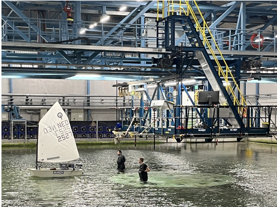
Figure 5.3: The carriage following the Optimist,, containing the Optotrak Certus HD and communication hardware.
