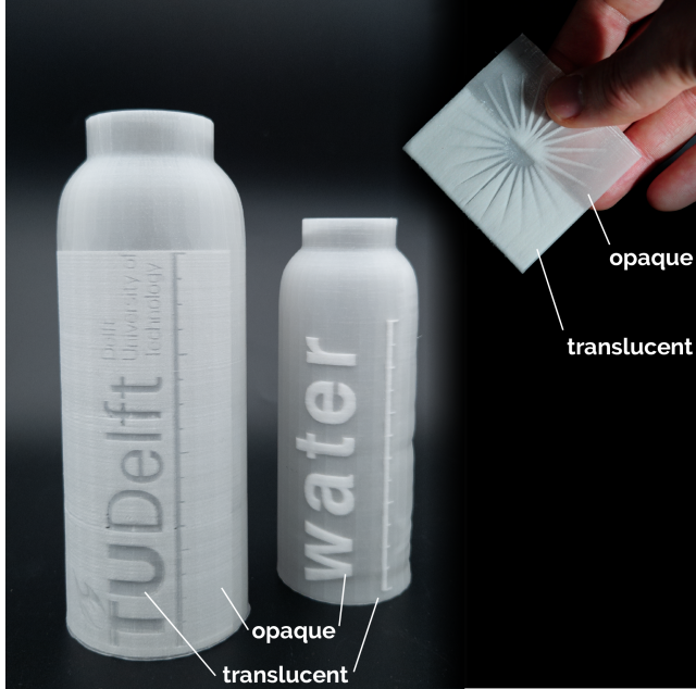
Figure 6: Liquid containers printed using "natural color" LW-PLA. Regions ironed at a low speed become opaque, while regions ironed at a high speed remain translucent.
