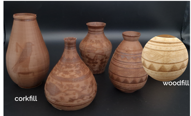
Figure 4: Examples showing local shade variations. Each object was printed using a single material; either Corkfill or Woodfill was used.
